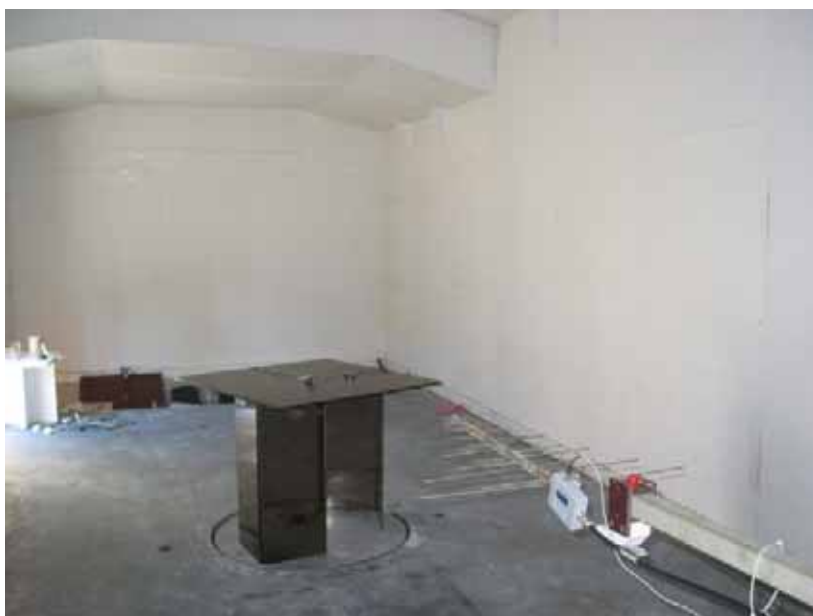
Radiated Emissions Measurement in Open Area Test Site Frequency range: 200 MHz – 1 GHz Configuration: WDP318 connected to charger and earphone
