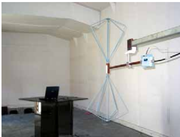
Radiated Emissions Measurement in Open Area Test Site Frequency range: 30 MHz – 200 MHz Configuration: WDP318 connected to laptop PC and earphone
