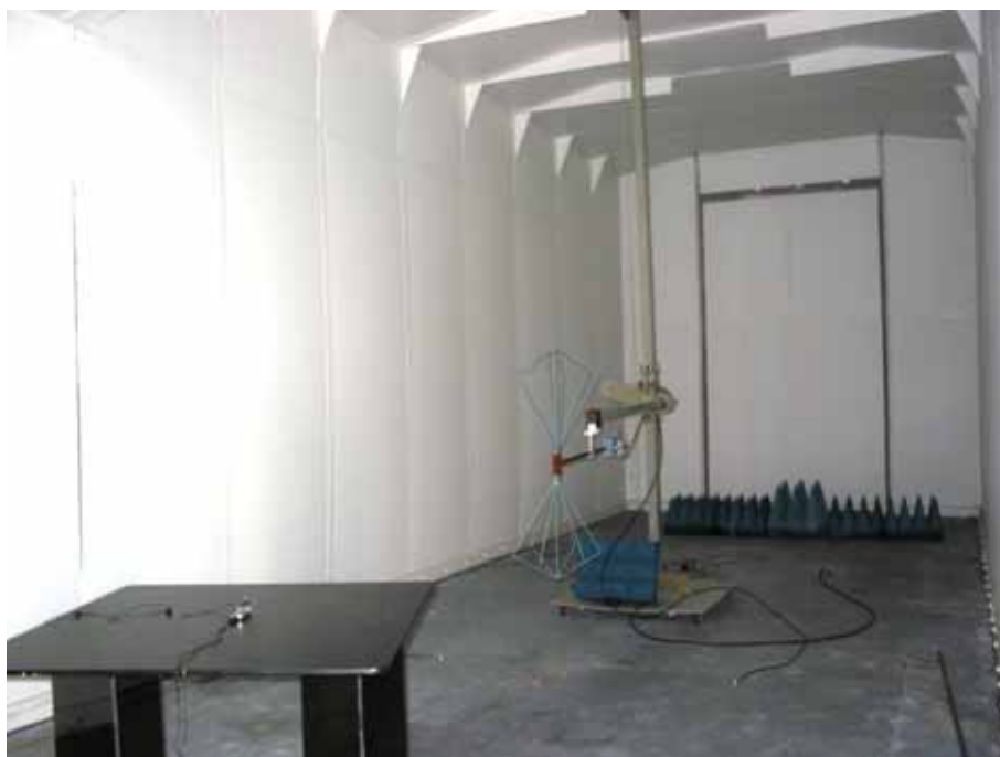
Radiated Emissions Measurement in Open Area Test Site Frequency range: 30 MHz – 200 MHz Configuration: WDP318 connected to charger and earphone
