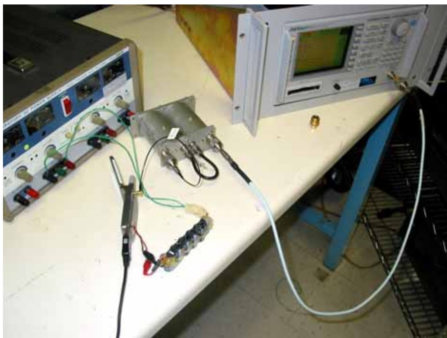
GSM 850/PCS 1900 Cellular Phone WDP318 Testing Out of Band Emissions at the Antenna Port using Notch Filter
