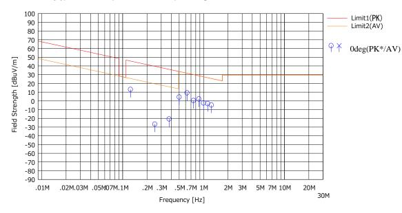
\* Data above 490 kHz were measured using a QP detector.
