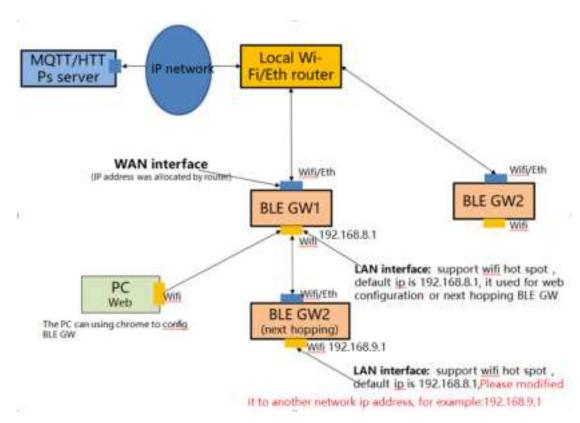
As shown above, each base station has two interfaces with different IP addresses. One of these IP addresses (referred to as the WAN port) is used to connect to the internet network (MQTT server), which has a series of firewall rule protection. The other IP address (referred to as LAN port, also known as the intranet interface) is used for Wi-Fi hotspot broadcasting.
