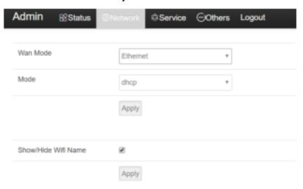
The IP address can be assigned in DHCP or static configuration.
