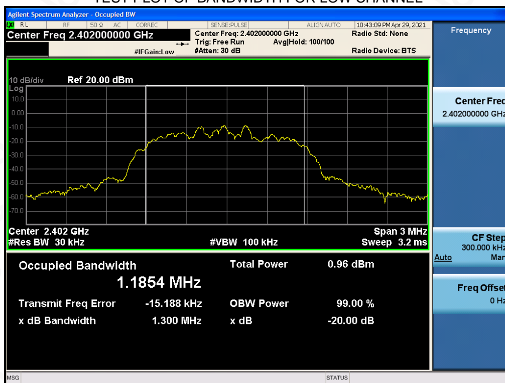
TEST PLOT OF BANDWIDTH FOR LOW CHANNEL
