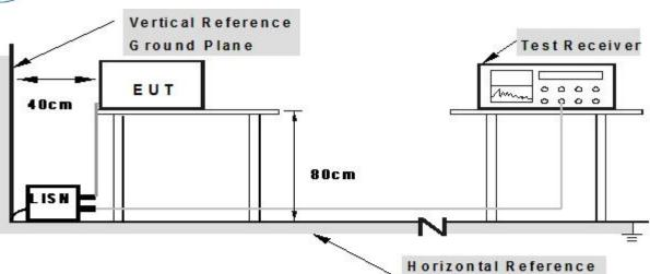
Note: 1. Support units were connected to second LISM. 2.Both of LISMs (AMM) are 80 cm from EUT and at least 80 from other units and other metal planes
