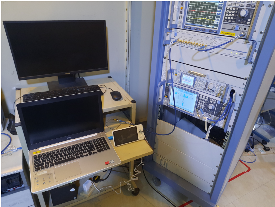
Conducted RF Output Power Test Setup
