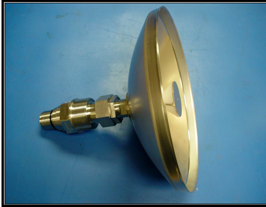
Photograph 39: 33 dBi Parabolic Antenna Side View
