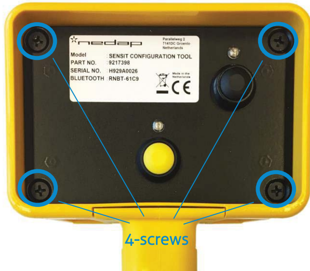
Figure 18: Configuration tool remove screws to open housing
