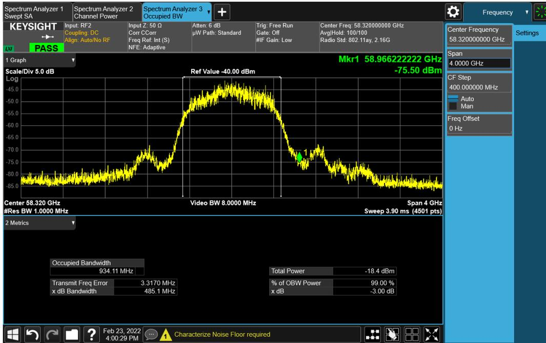
**Occupied Channel Bandwidth Low Channel 1 GHz Bandwidth**
