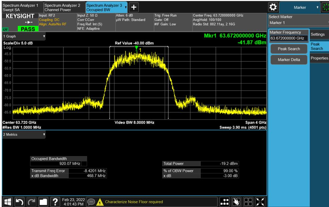
**Occupied Channel Bandwidth Mid Channel 1 GHz Bandwidth**
