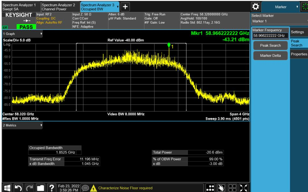
**Occupied Channel Bandwidth Low Channel 2 GHz Bandwidth**
