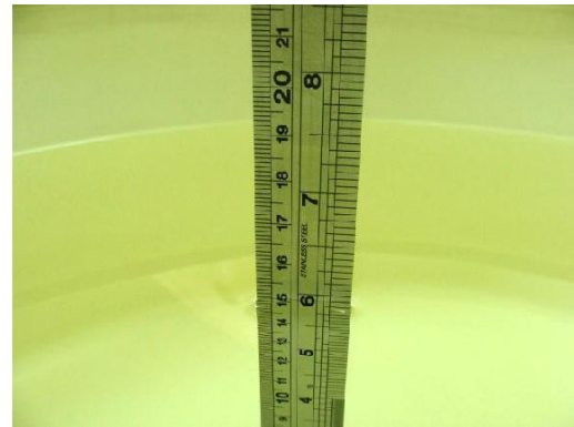
Fig 7.2 Photo of Liquid Height for Body SAR
