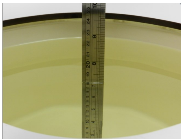
Fig 10.2 Photo of Liquid Height for Body SAR
