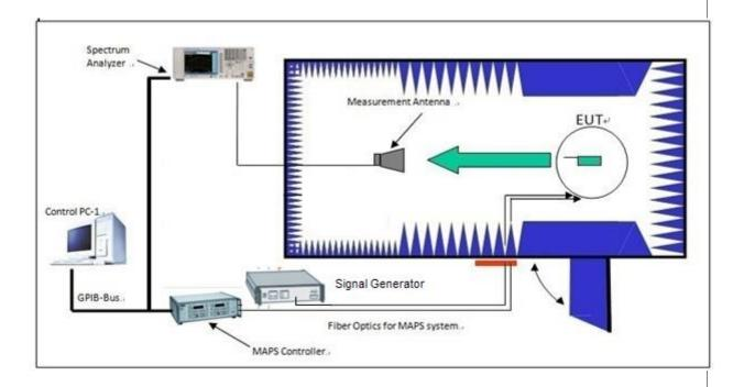
Figure 1. 2D antenna pattern test system.
