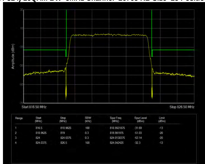
Band26(814-824) QPSK BW=1.4MHz Channel=26697 RB Size=1 Position=#0 Extended
