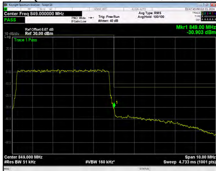
Band26(824-849) QPSK BW=1.4MHz Channel=26797 RB Size=1 Position=#0 Extended
