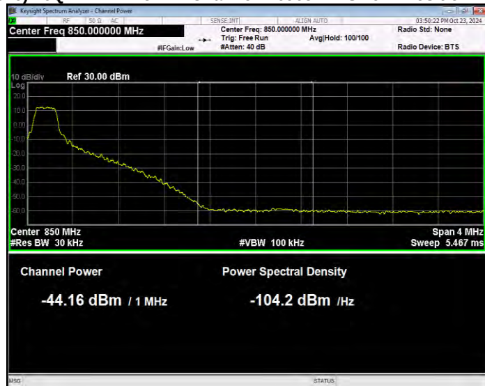
Band26(824-849) 16QAM BW=15MHz Channel=26965 RB Size=1 Position=#Max Normal
