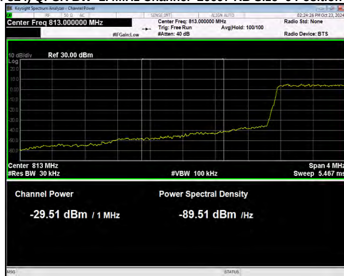
Band26(814-824) QPSK BW=1.4MHz Channel=26697 RB Size=6 Position=#0 Normal
