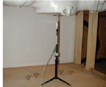
Figure 9.1 Dipole Verification Test Setup Diagram & Photo
