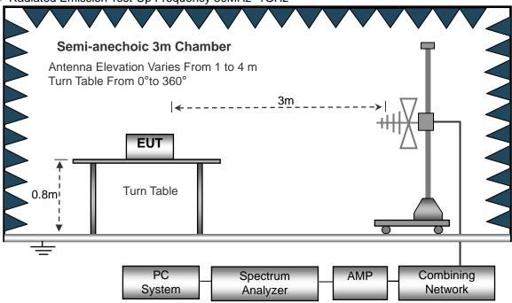
(C) Radiated Emission Test-Up Frequency Above 1GHz
