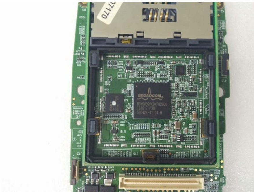
EUT – IC Chip View
