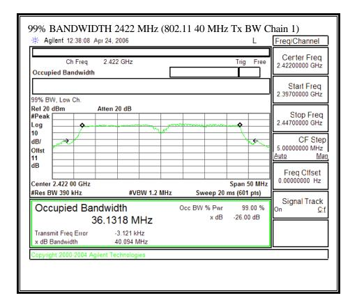
EUT: BROADCOM 802.11ag /DRAFT 802.11n WIRELESS LAN PCI-E MINI CARD
