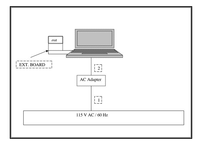
EUT: BROADCOM 802.11ag /DRAFT 802.11n WIRELESS LAN PCI-E MINI CARD
