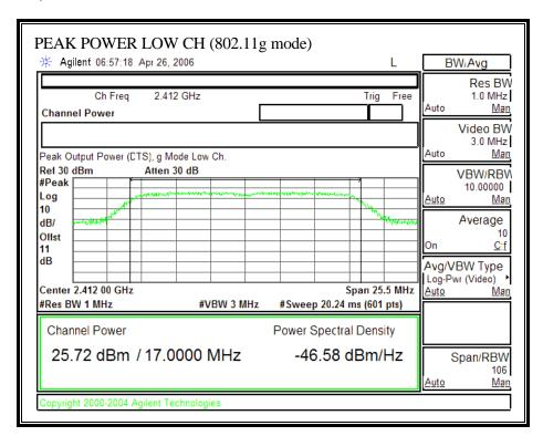
EUT: BROADCOM 802.11ag /DRAFT 802.11n WIRELESS LAN PCI-E MINI CARD
