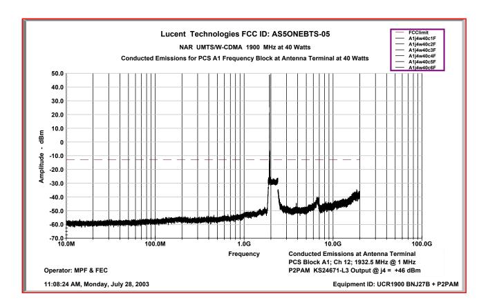
Conducted Emissions Characteristics Block A3 UMTS1900 Ch 62; 1942.5 MHz at Tx Antenna Terminal at +46 dBm per single 5 MHz carrier
