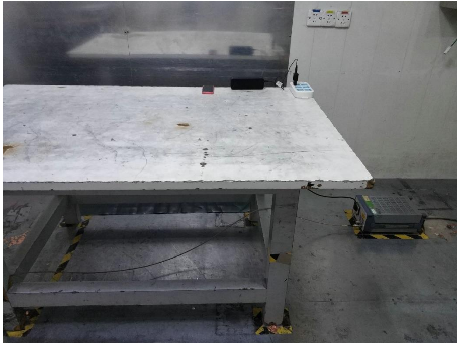
Photograph 1: Set-up for Conducted Emission on AC Mains
