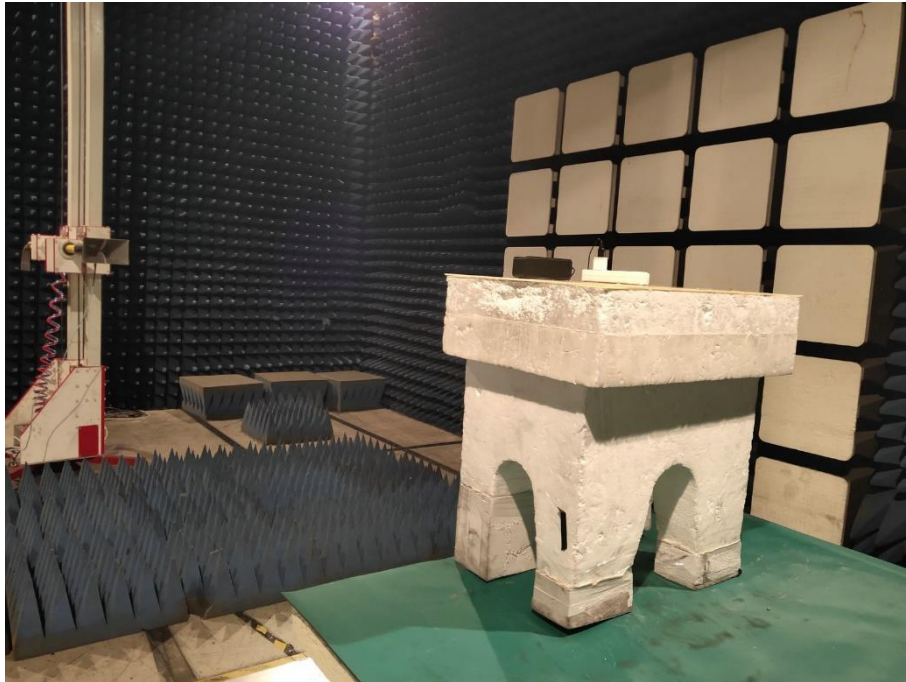
Photograph 3: Set-up for Radiated Spurious Emission, Above 1GHz
