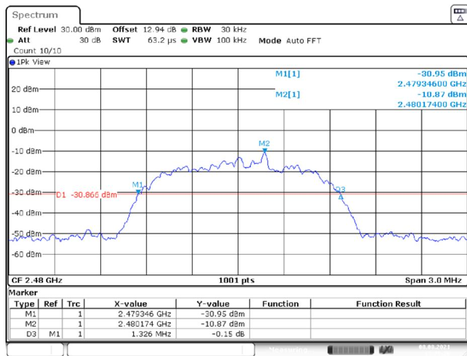
**99% OCCUPIED BANDWIDTH****DH5\_2402MHz**
