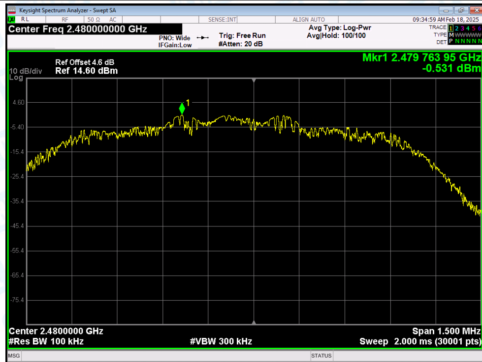
Tx. Spurious NVNT 3-DH1 2480MHz Ant1 Emission
