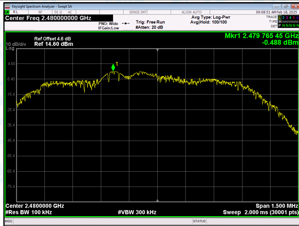
Tx. Spurious NVNT 2-DH1 2480MHz Ant1 Emission
