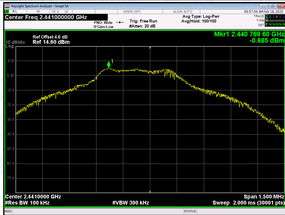
Tx. Spurious NVNT 1-DH1 2441MHz Ant1 Emission
