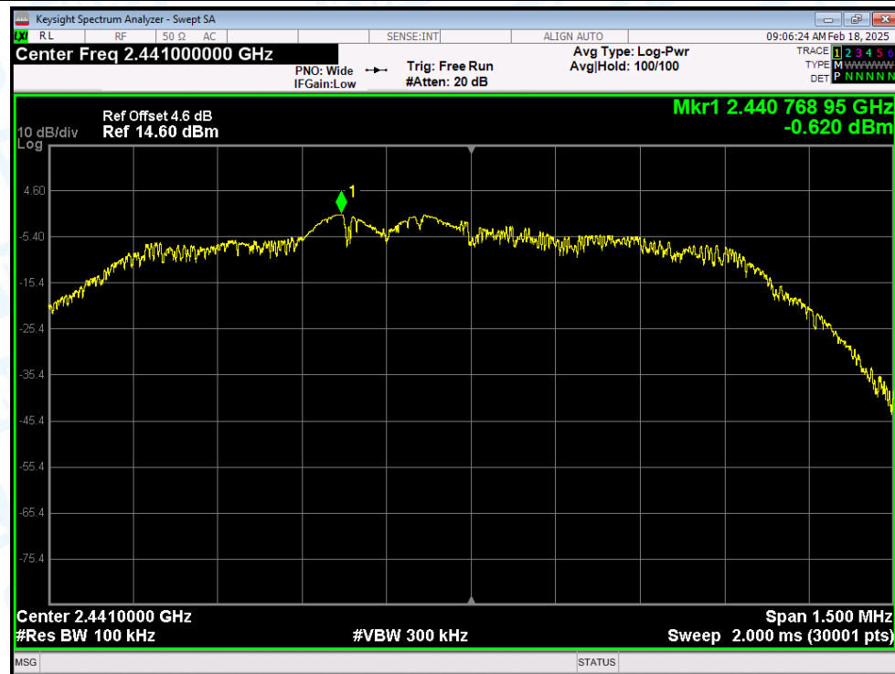
Tx. Spurious NVNT 2-DH1 2441MHz Ant1 Emission
