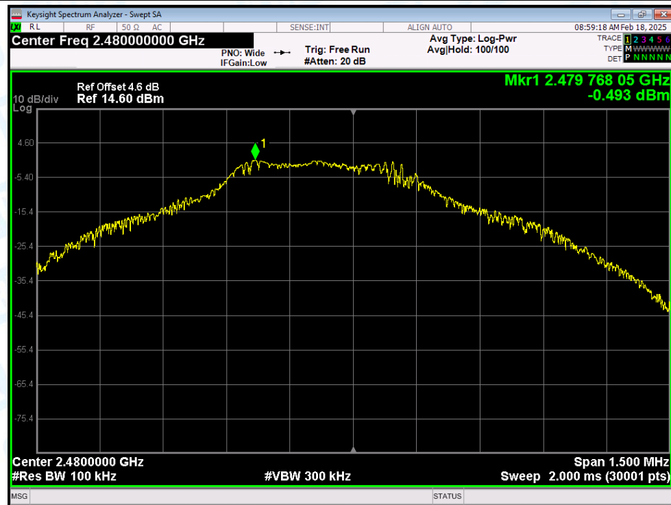
Tx. Spurious NVNT 1-DH1 2480MHz Ant1 Emission
