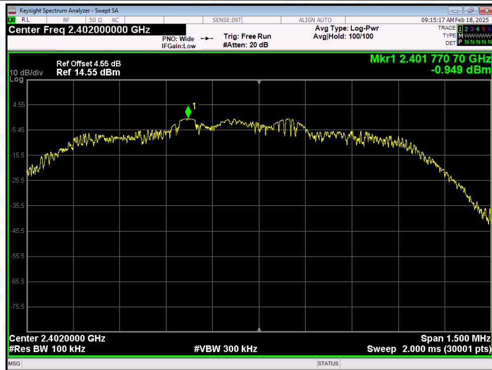
Tx. Spurious NVNT 3-DH1 2402MHz Ant1 Emission
