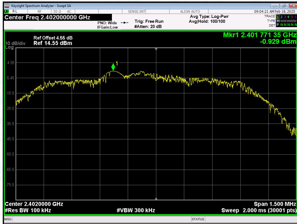
Tx. Spurious NVNT 2-DH1 2402MHz Ant1 Emission
