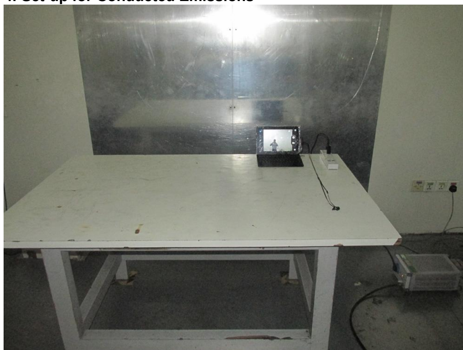
Photograph 4: Set-up for Conducted Emissions
