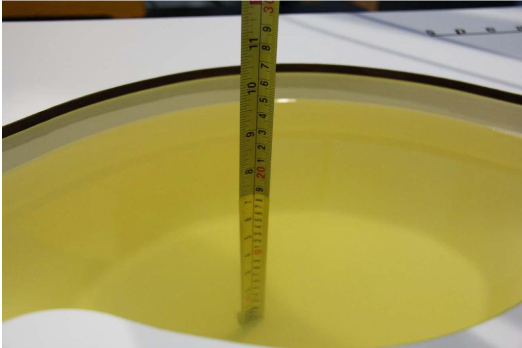
Picture 7-1: Liquid depth in the Flat Phantom(2450MHz)
