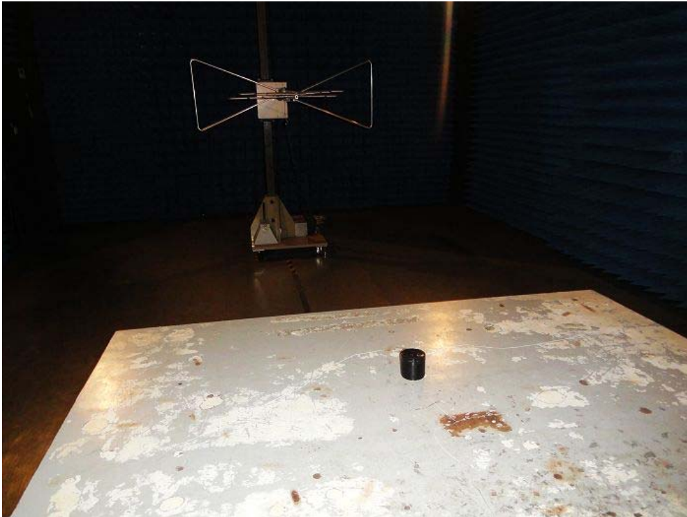
Radiated Emission Test Setup:
