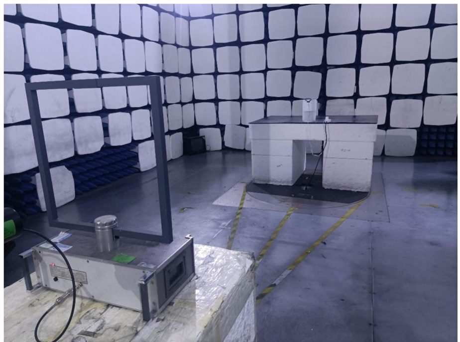
Radiation Emission Test Setup (Below 30MHz)
