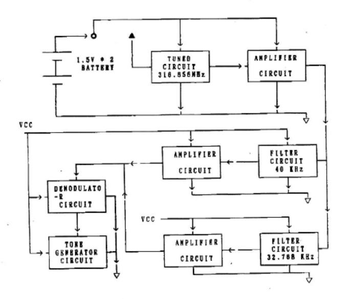
The signal is received from the antenna, the input signal is tuned by tuned circuit at 316.656 MBz. the signal is through amplifier circuit, filter circuit, demodulator circuit. At last, into tone generator to produce voice.
