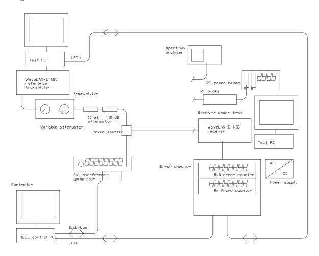
Figure 1, measurement test set-up.
