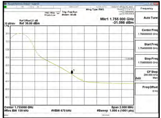
EDGE B4 15M CH20325 QPSK(1,74)
