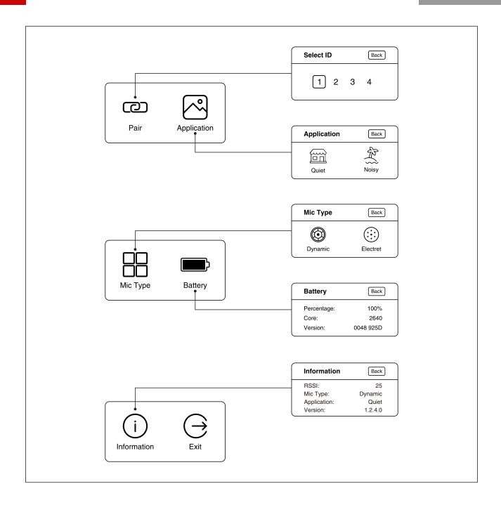
Long press the "OK" button for about three seconds to enter the root menu, select the menu and press "OK" to enter the next level. Each menu feature is described as follows.
