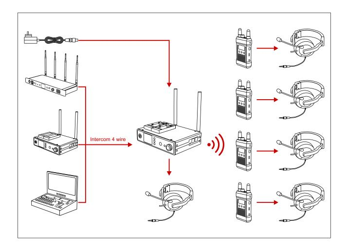
The base station of this wireless full-duplex intercom system supports up to 4 beltpacks. The base station and the beltpacks support dynamic and electret mics. They could be switched by selecting different applications in the menu. The 4-pin audio interface on the base station enables the device to connect with other audio systems, which can increase the quantity of beltpacks and also the wireless communication range.
