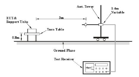
The radiated emission tests were performed in the 3-meter chamber test site, using the setup accordance with the ANSI C63.10-2013 and RSS-Gen. The specification used was the FCC Part Subpart C and the RSS-210 and RSS-Gen limits.
