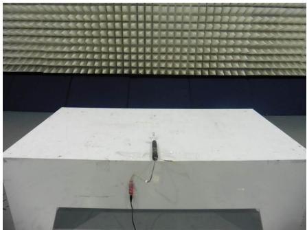
Electromagnetic Radiated Disturbance Setup Photograph
