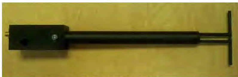
Figure 1 – MVG COMOSAR Validation Dipole
