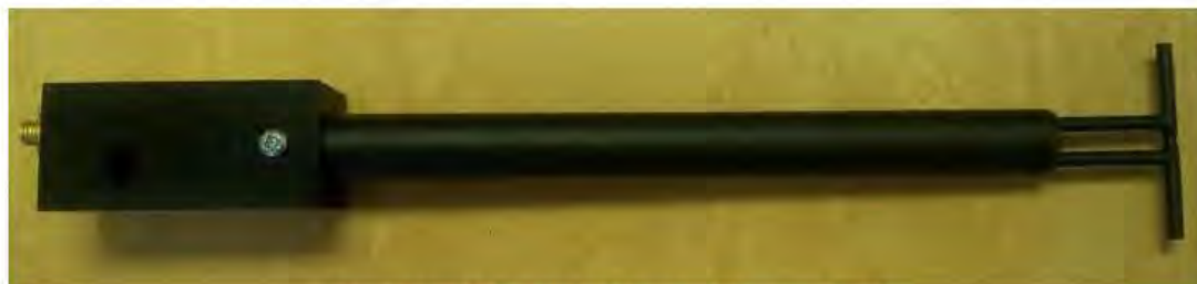
Figure 1 – MVG COMOSAR Validation Dipole
