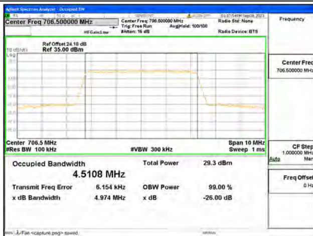
B17 / 5MHz / 64QAM/ Low CH
