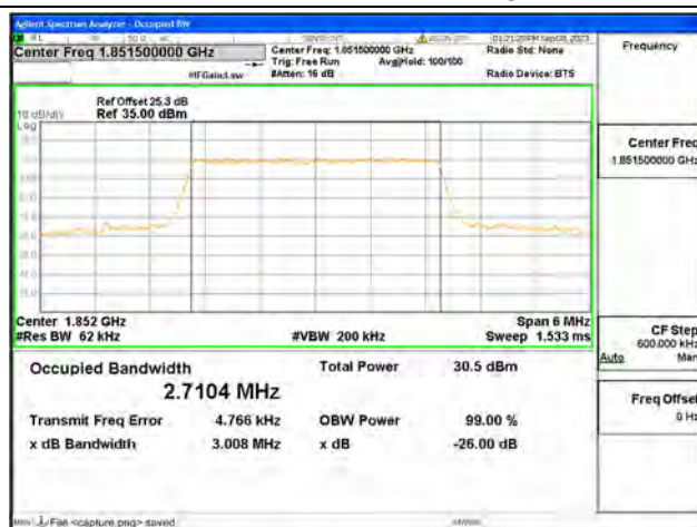
B25 / 3MHz / 16QAM/ Low CH
