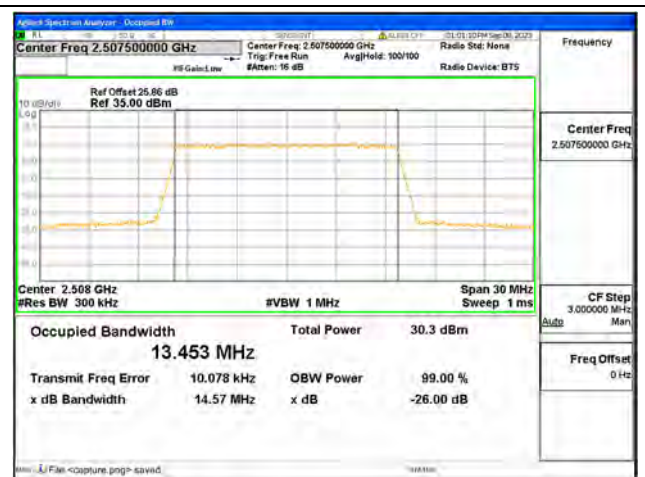
B7 / 15MHz / 16QAM/ Low CH
