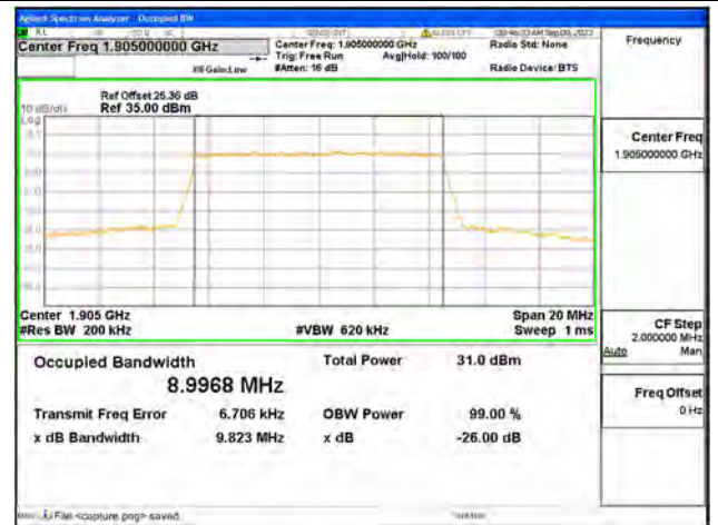
B2 / 10MHz / QPSK/ High CH
