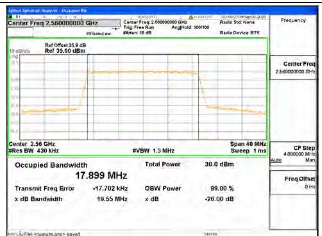
B7 / 20MHz / 64QAM/ High CH
