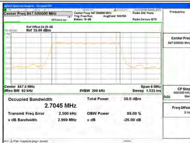
B5 / 3MHz / 16QAM/ High CH
