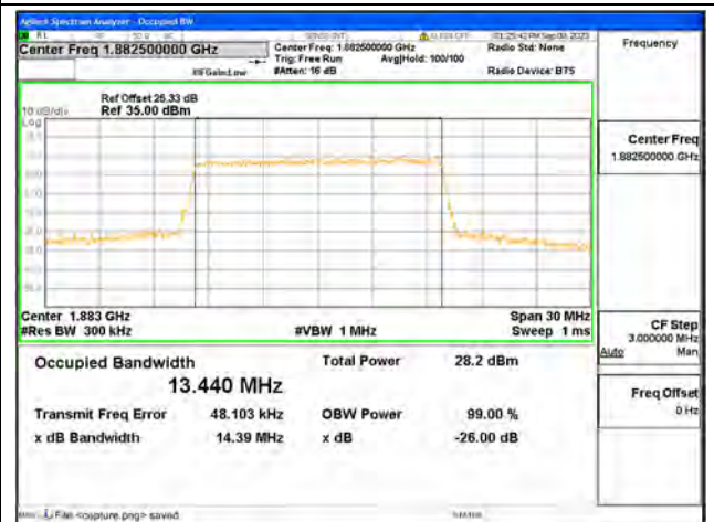
B25 / 15MHz / 64QAM/ Mid CH
