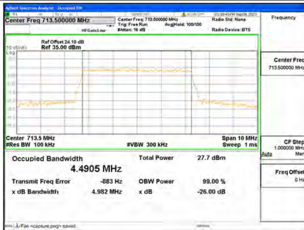
B17 / 5MHz / 64QAM/ High CH
