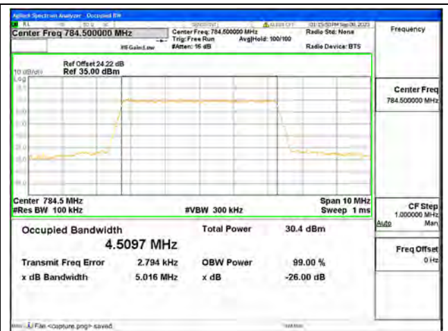
B13 / 5MHz / 16QAM/ High CH
