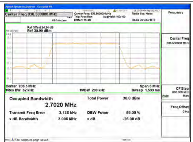
B5 / 3MHz / 16QAM/ Mid CH
