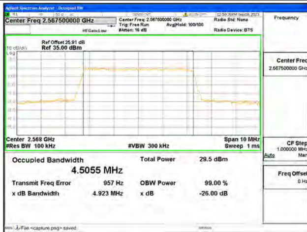
B7 / 5MHz / 64QAM/ High CH
