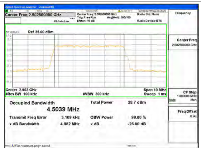
B7 / 5MHz / 16QAM/ Low CH
