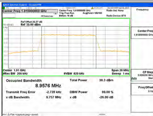
B25 / 10MHz / 16QAM/ High CH
