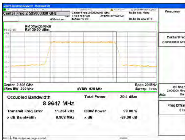
B7 / 10MHz / 16QAM/ Low CH
