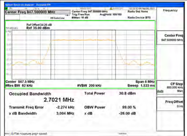
B5 / 3MHz / QPSK/ High CH
