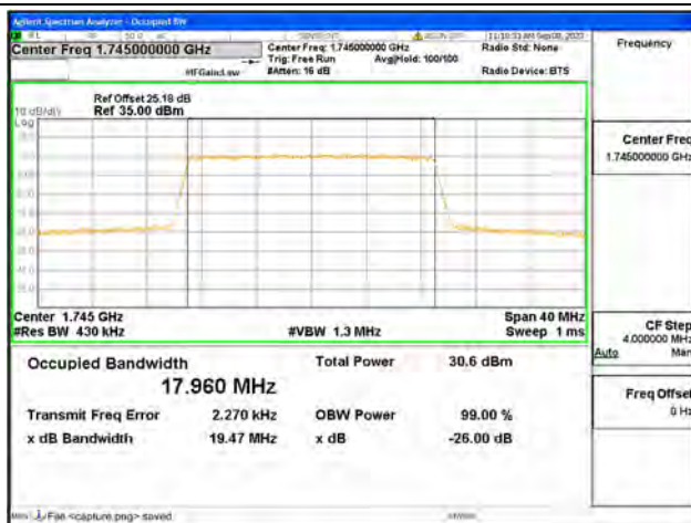
B4 / 20MHz / 16QAM/ High CH
