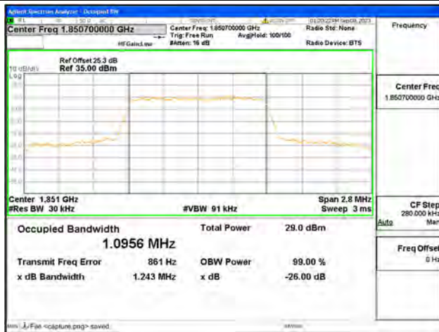
B25 / 1.4MHz / 64QAM/ Low CH
