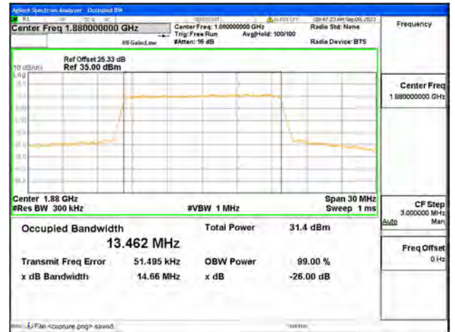
B2 / 15MHz / QPSK/ Mid CH
