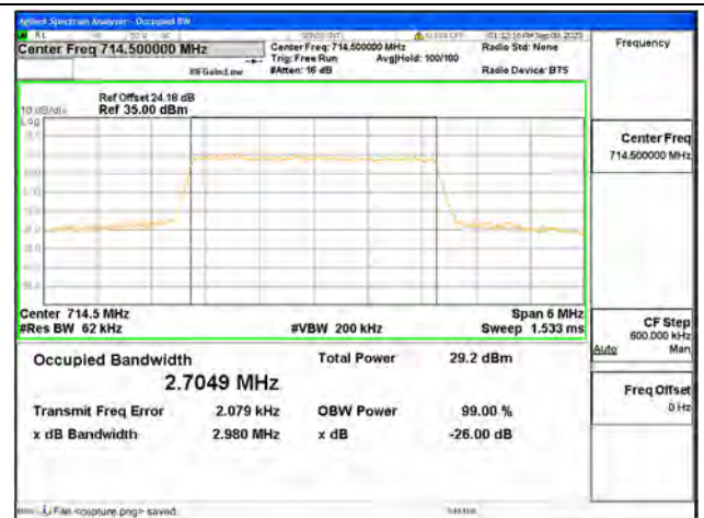
B12 / 3MHz / 64QAM/ High CH
