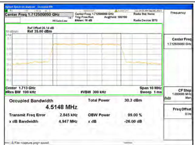
B4 / 5MHz / 16QAM/ Low CH
