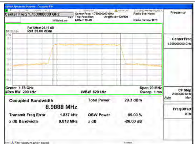
B4 / 10MHz / 64QAM/ High CH
