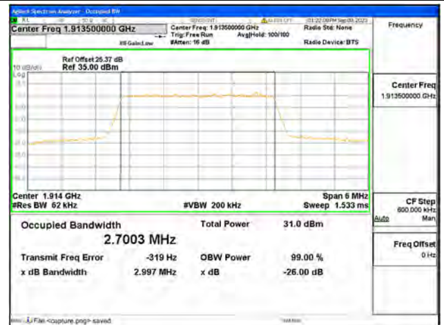
B25 / 3MHz / QPSK/ High CH
