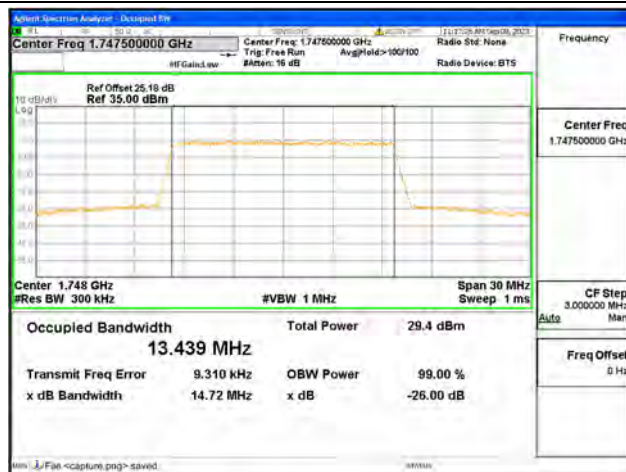
B4 / 15MHz / 64QAM/ High CH
