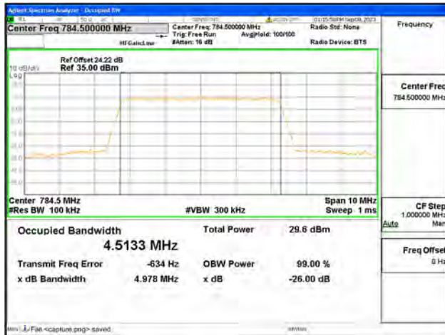
B13 / 5MHz / 64QAM/ High CH
