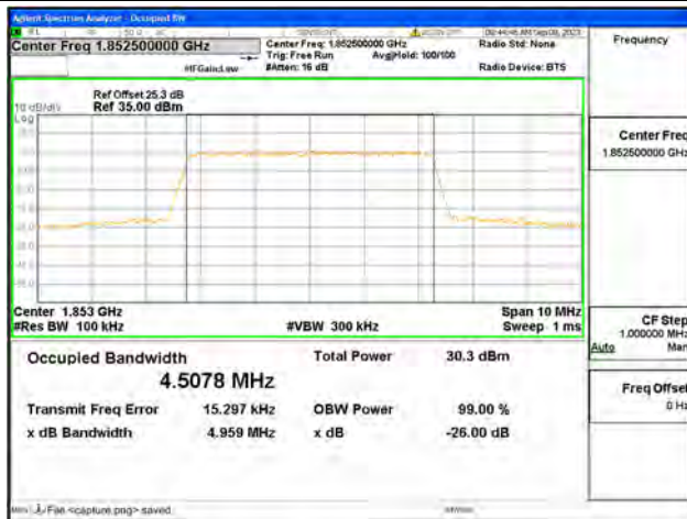
B2 / 5MHz / 64QAM/ Low CH
