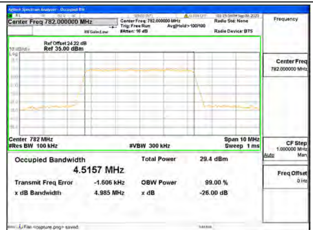
B13 / 5MHz / 64QAM/ Mid CH
