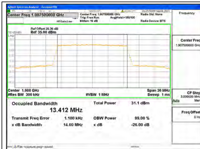
B25 / 15MHz / QPSK/ High CH
