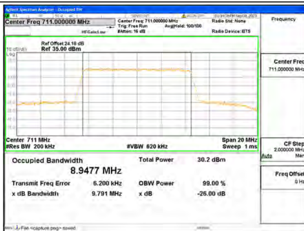
B12 / 10MHz / 16QAM/ High CH
