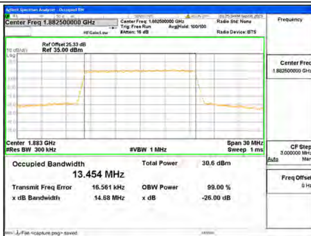
B25 / 15MHz / 16QAM/ Mid CH
