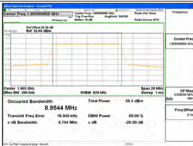
B2 / 10MHz / 16QAM/ High CH
