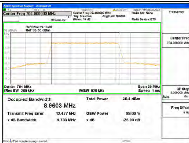
B12 / 10MHz / 16QAM/ Low CH
