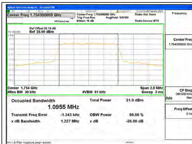
B4 / 1.4MHz / QPSK/ High CH
