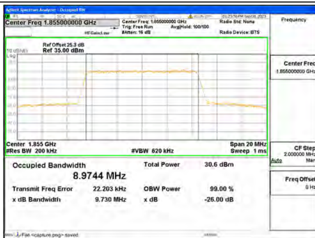
B25 / 10MHz / 16QAM/ Low CH
