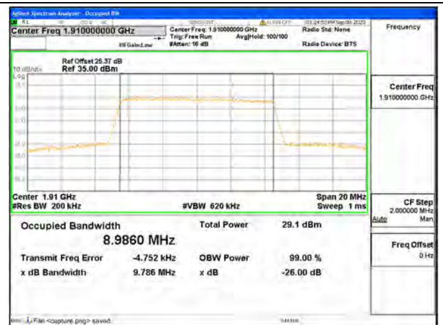
B25 / 10MHz / 64QAM/ High CH
