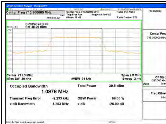
B12 / 1.4MHz / QPSK/ High CH
