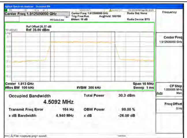
B25 / 5MHz / 16QAM/ High CH
