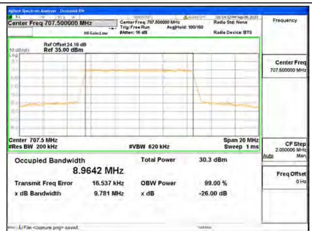
B12 / 10MHz / 16QAM/ Mid CH
