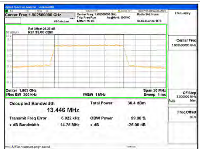
B2 / 15MHz / 16QAM/ High CH
