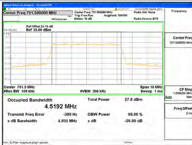
B12 / 5MHz / 64QAM/ Low CH
