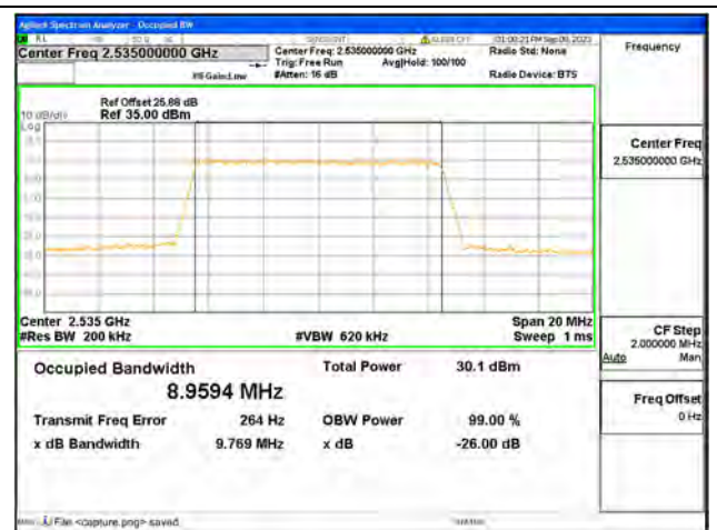
B7 / 10MHz / 16QAM/ Mid CH
