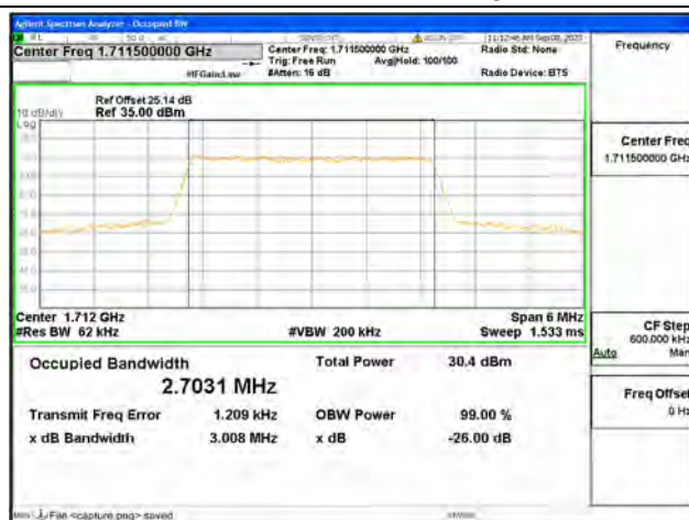
B4 / 3MHz / 16QAM/ Low CH
