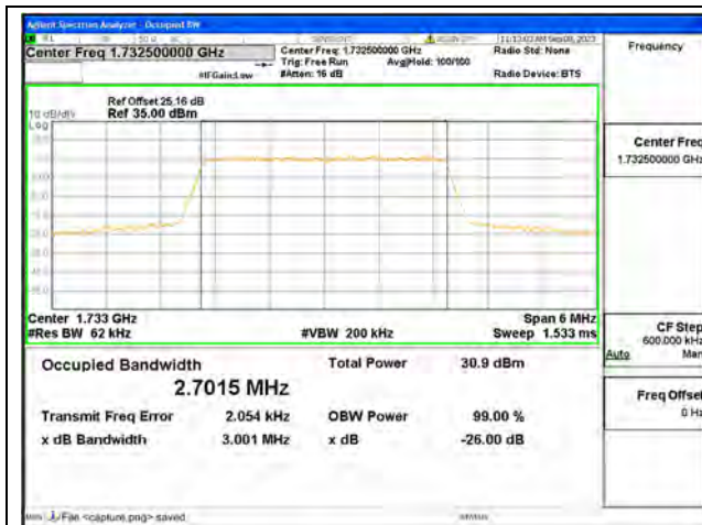
B4 / 3MHz / QPSK/ Mid CH
