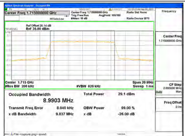
B4 / 10MHz / 64QAM/ Low CH
