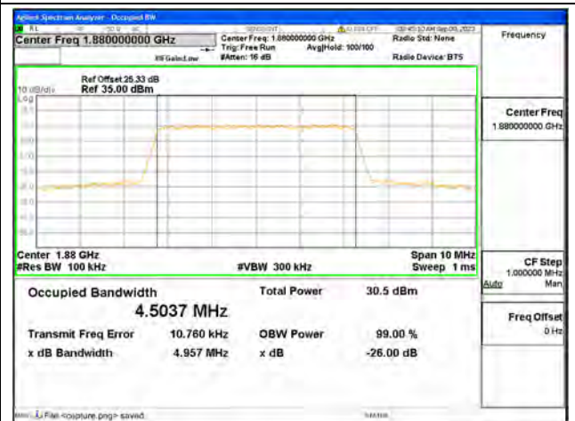
B2 / 5MHz / 64QAM/ Mid CH
