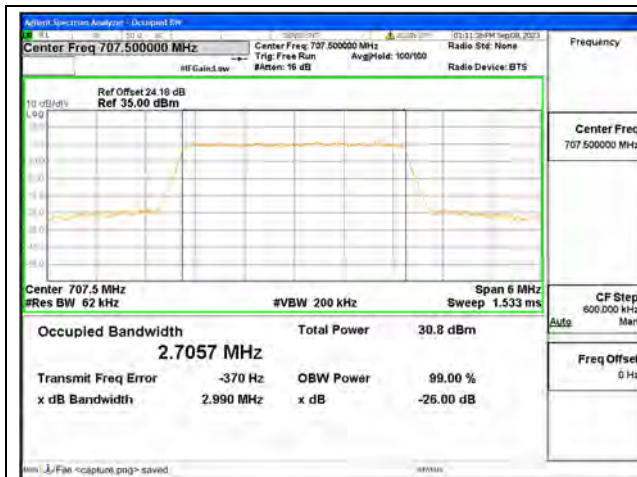
B12 / 3MHz / QPSK/ Mid CH
