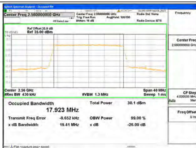
B7 / 20MHz / 16QAM/ High CH
