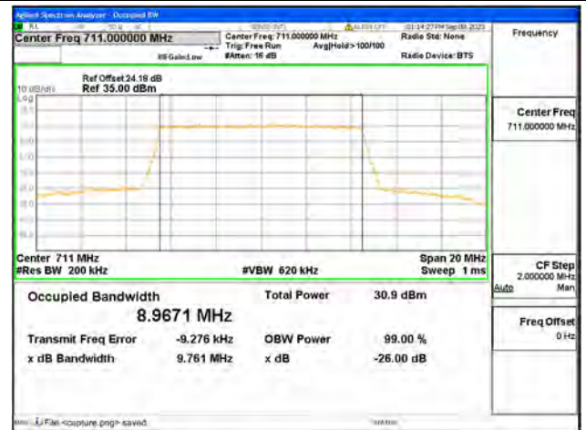
B12 / 10MHz / QPSK/ High CH
