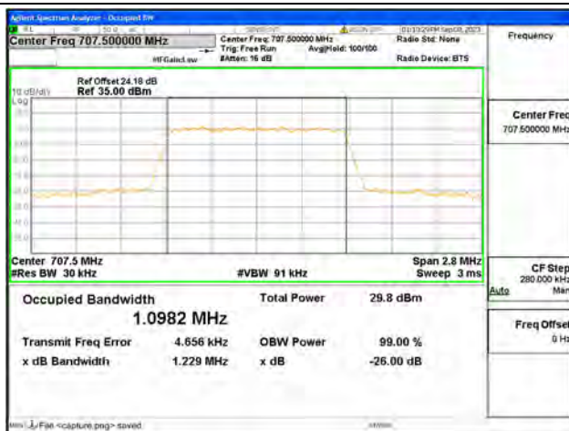
B12 / 1.4MHz / 16QAM/ Mid CH
