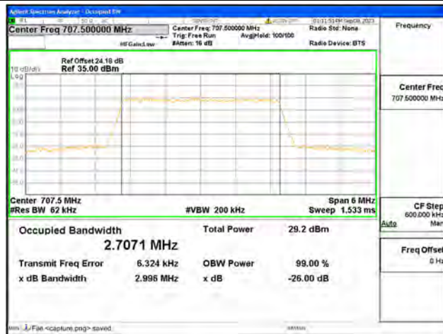
B12 / 3MHz / 64QAM/ Mid CH
