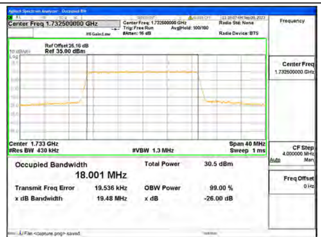
B4 / 20MHz / 16QAM/ Mid CH
