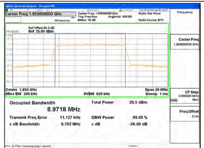
B25 / 10MHz / 64QAM/ Low CH
