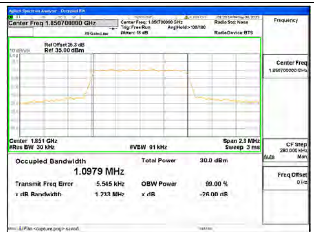
B25 / 1.4MHz / 16QAM/ Low CH
