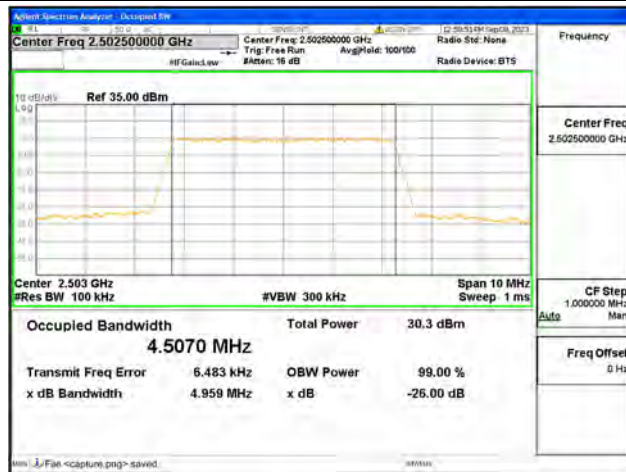
B7 / 5MHz / 64QAM/ Low CH
