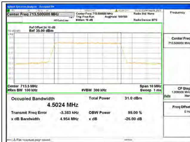
B12 / 5MHz / QPSK/ High CH
