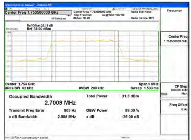
B4 / 3MHz / QPSK/ High CH
