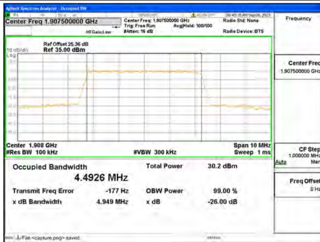
B2 / 5MHz / 64QAM/ High CH
