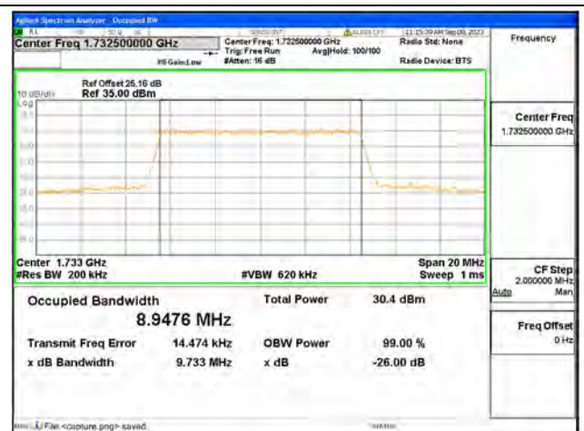
B4 / 10MHz / 16QAM/ Mid CH
