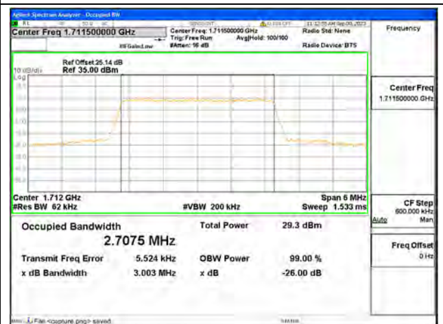
B4 / 3MHz / 64QAM/ Low CH
