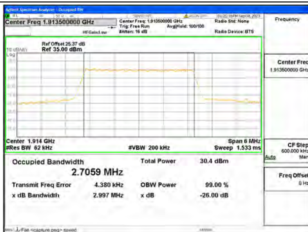
B25 / 3MHz / 16QAM/ High CH
