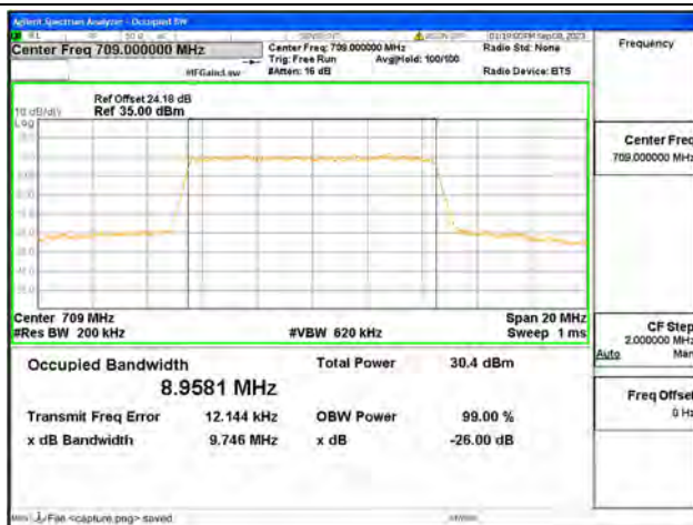
B17 / 10MHz / 16QAM/ Low CH
