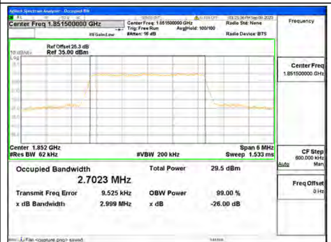
B25 / 3MHz / 64QAM/ Low CH
