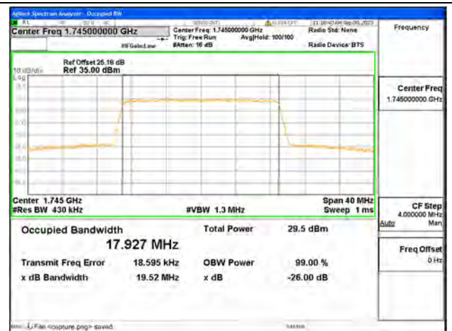
B4 / 20MHz / 64QAM/ High CH
