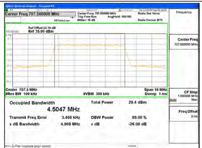
B12 / 5MHz / 64QAM/ Mid CH
