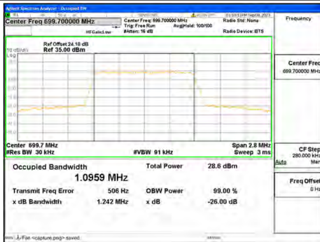
B12 / 1.4MHz / 64QAM/ Low CH
