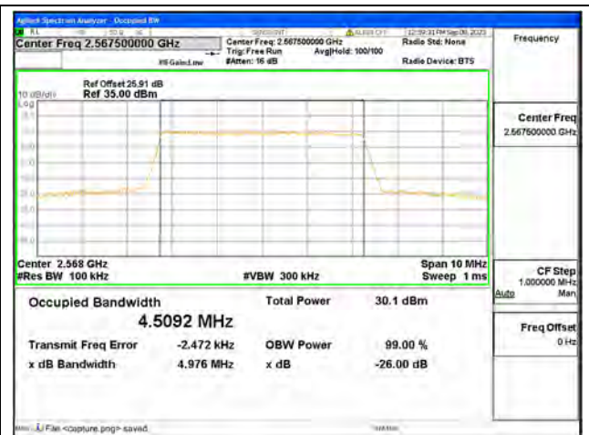
B7 / 5MHz / 16QAM/ High CH
