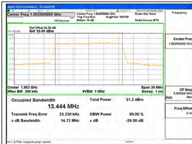
B2 / 15MHz / QPSK/ High CH
