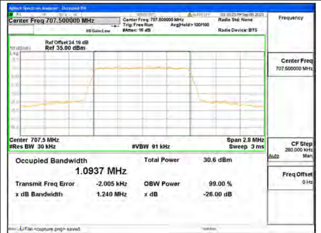
B12 / 1.4MHz / QPSK/ Mid CH
