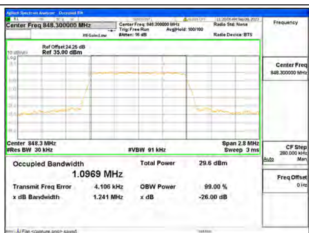
B5 / 1.4MHz / 16QAM/ High CH
