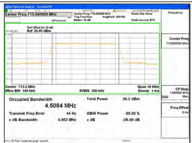
B12 / 5MHz / 16QAM/ High CH
