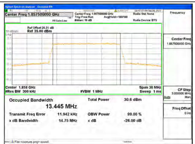
B2 / 15MHz / 16QAM/ Low CH
