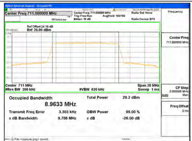
B12 / 10MHz / 64QAM/ High CH
