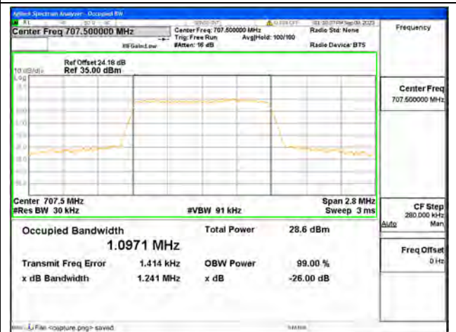
B12 / 1.4MHz / 64QAM/ Mid CH
