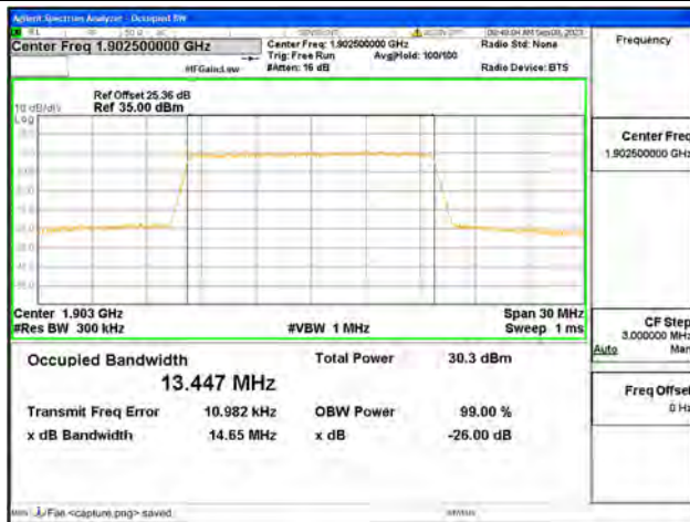
B2 / 15MHz / 64QAM/ High CH
