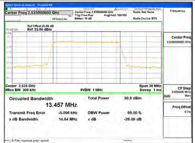
B7 / 15MHz / QPSK/ Mid CH
