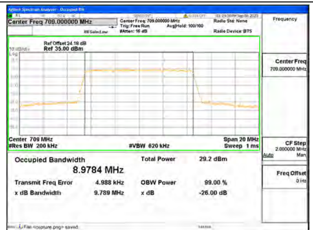
B17 / 10MHz / 64QAM/ Low CH
