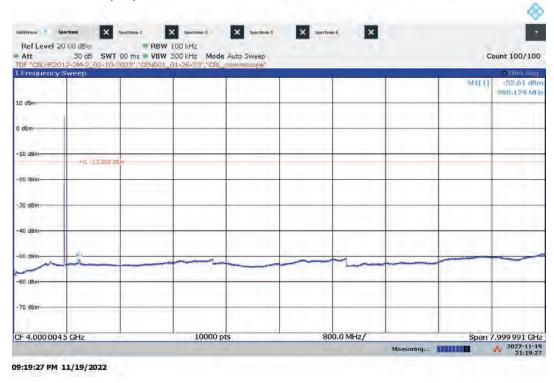
Hi-PIM Antenna Port Conducted Emissions, 9 kHz-8 GHz Worst-case output power: Bandwidth: 5 MHz, Modulation: 64QAM, ANT0, Mid Channel
