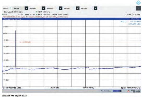
Hi-PIM Antenna Port Conducted Emissions, 9 kHz-8 GHz Worst-case output power: Bandwidth: 5 MHz, Modulation: 64QAM, ANT1, Mid Channel
