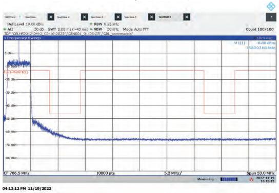
Lo-PIM – ANTO Mid Channel Emission/Band Edge (Mask e (3)) Bandwidth: 5 MHz, Modulation: 64QAM
