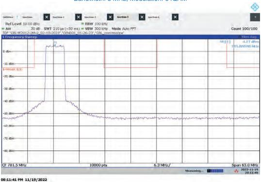
Hi-PIM – ANTO High Channel Emission/Band Edge (Mask e (1)) Bandwidth: 5 MHz, Modulation: 64QAM
