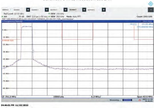
Lo-PIM – ANTO Mid Channel Emission/Band Edge (Mask e (1)) Bandwidth: 5 MHz, Modulation: 256QAM
