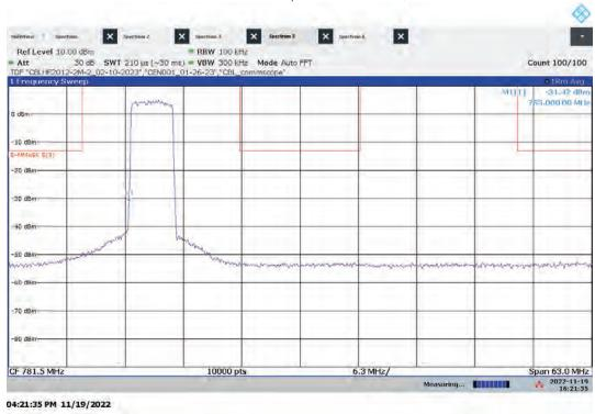
Lo-PIM – ANTO Low Channel Emission/Band Edge (Mask e (1)) Bandwidth: 5 MHz, Modulation: 256QAM
