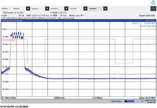
Hi-PIM – ANTO High Channel Emission/Band Edge (Mask e (3)) Bandwidth: 5 MHz, Modulation: 16QAM
