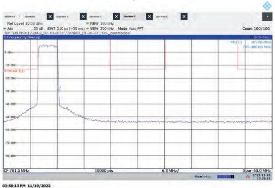
Lo-PIM – ANT1 Low Channel Emission/Band Edge (Mask e (3)) Bandwidth: 5 MHz, Modulation: 64QAM
