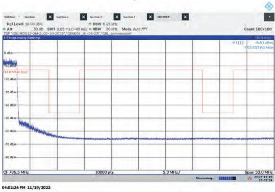
Lo-PIM – ANTO Low Channel Emission/Band Edge (Mask e (3)) Bandwidth: 5 MHz, Modulation: 64QAM
