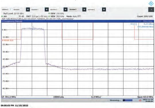
Hi-PIM – ANTO Low Channel Emission/Band Edge (Mask e (1)) Bandwidth: 5 MHz, Modulation: QPSK
