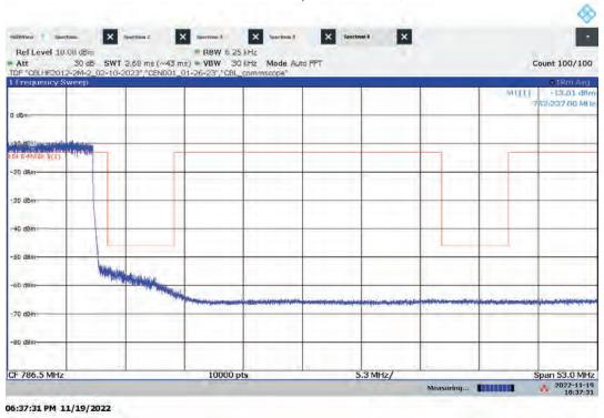
Hi-PIM – ANT0 High Channel Emission/Band Edge (Mask e (3)) Bandwidth: 10 MHz, Modulation: QPSK
