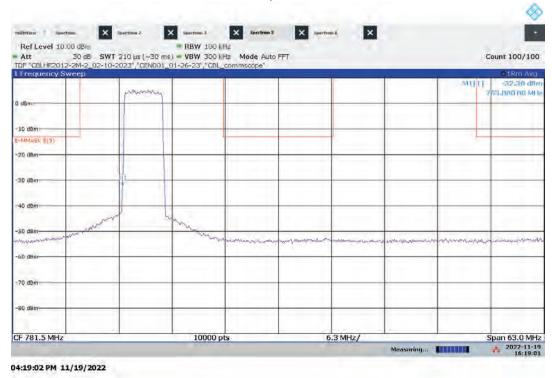
Lo-PIM – ANT1 High Channel Emission/Band Edge (Mask e (3)) Bandwidth: 5 MHz, Modulation: 64QAM
