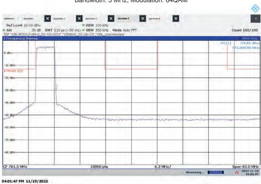
Lo-PIM – ANTO Mid Channel Emission/Band Edge (Mask e (1)) Bandwidth: 5 MHz, Modulation: 64QAM
