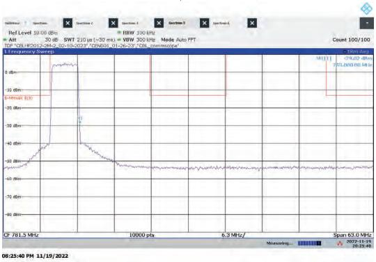
Hi-PIM – ANT0 Mid Channel Emission/Band Edge (Mask e (1)) Bandwidth: 5 MHz, Modulation: 256QAM
