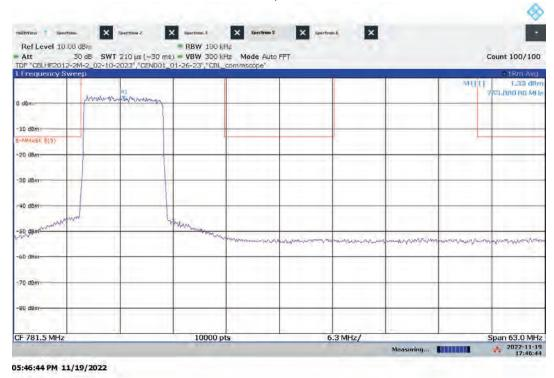
Lo-PIM – ANT1 High Channel Emission/Band Edge (Mask e (3)) Bandwidth: 10 MHz, Modulation: 64QAM
