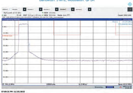
Hi-PIM – ANTO Mid Channel Emission/Band Edge (Mask e (1)) Bandwidth: 5 MHz, Modulation: QPSK
