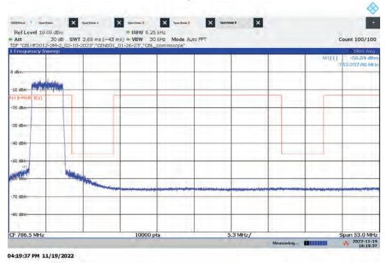
Lo-PIM – ANT1 High Channel Emission/Band Edge (Mask e (1)) Bandwidth: 5 MHz, Modulation: 64QAM
