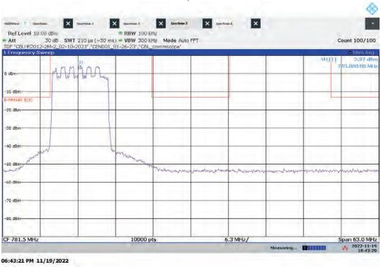
Hi-PIM – ANTO High Channel Emission/Band Edge (Mask e (1)) Bandwidth: 10 MHz, Modulation: 64QAM
