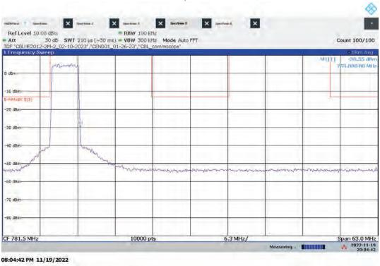
Hi-PIM – ANTO Mid Channel Emission/Band Edge (Mask e (1)) Bandwidth: 5 MHz, Modulation: 64QAM
