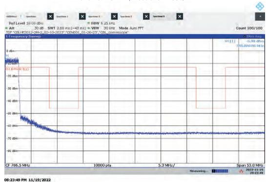
Hi-PIM – ANT1 Low Channel Emission/Band Edge (Mask e (1)) Bandwidth: 5 MHz, Modulation: 256QAM
