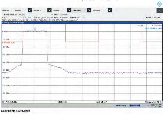
Hi-PIM – ANTO High Channel Emission/Band Edge (Mask e (1)) Bandwidth: 10 MHz, Modulation: 16QAM
