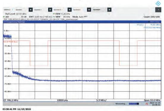
Lo-PIM – ANT1 Low Channel Emission/Band Edge (Mask e (1)) Bandwidth: 5 MHz, Modulation: 64QAM
