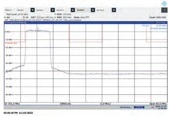
Lo-PIM – ANT1 High Channel Emission/Band Edge (Mask e (3)) Bandwidth: 10 MHz, Modulation: 256QAM
