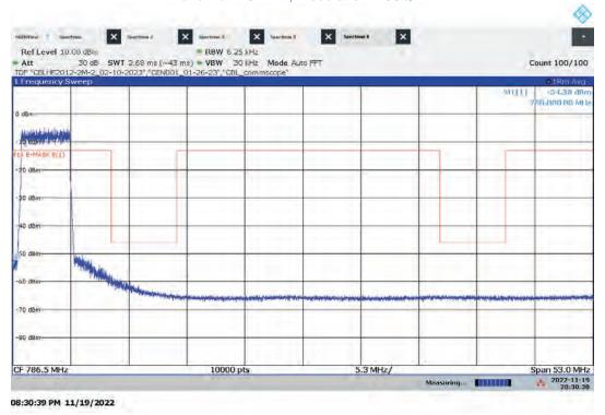
Hi-PIM – ANT1 Mid Channel Emission/Band Edge (Mask e (1)) Bandwidth: 5 MHz, Modulation: 256QAM
