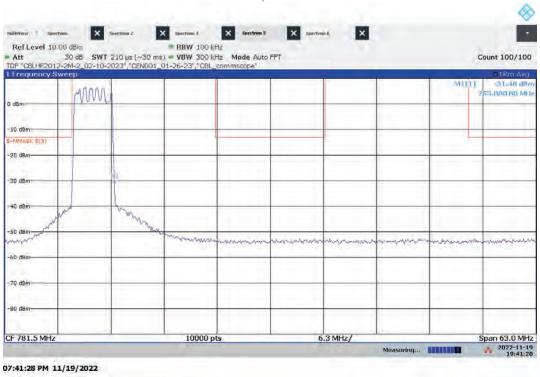
Hi-PIM – ANTO Mid Channel Emission/Band Edge (Mask e (1)) Bandwidth: 5 MHz, Modulation: 16QAM
