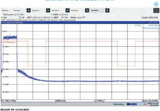
Hi-PIM – ANTO Mid Channel Emission/Band Edge (Mask e (3)) Bandwidth: 5 MHz, Modulation: 64QAM
