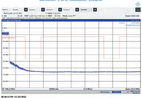
Hi-PIM – ANTO Low Channel Emission/Band Edge (Mask e (3)) Bandwidth: 5 MHz, Modulation: 256QAM
