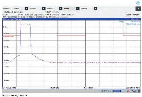
Hi-PIM – ANT1 Low Channel Emission/Band Edge (Mask e (3)) Bandwidth: 5 MHz, Modulation: 256QAM
