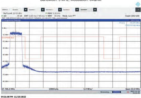
Lo-PIM – ANTO High Channel Emission/Band Edge (Mask e (3)) Bandwidth: 5 MHz, Modulation: 64QAM
