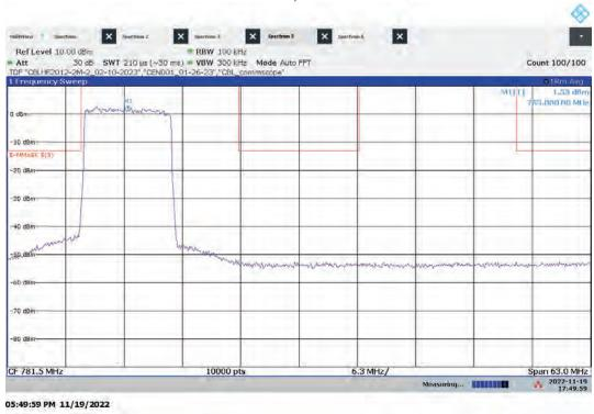
Lo-PIM – ANTO High Channel Emission/Band Edge (Mask e (1)) Bandwidth: 10 MHz, Modulation: 256QAM
