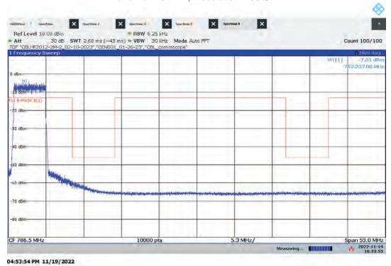
Lo-PIM – ANT1 Mid Channel Emission/Band Edge (Mask e (1)) Bandwidth: 5 MHz, Modulation: 256QAM
