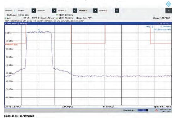
Hi-PIM – ANT1 High Channel Emission/Band Edge (Mask e (3)) Bandwidth: 10 MHz, Modulation: 256QAM
