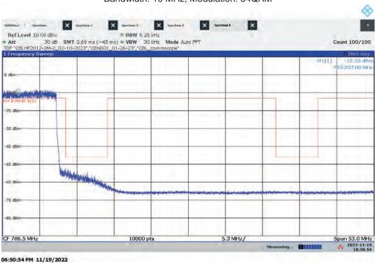
Hi-PIM – ANTO High Channel Emission/Band Edge (Mask e (3)) Bandwidth: 10 MHz, Modulation: 64QAM
