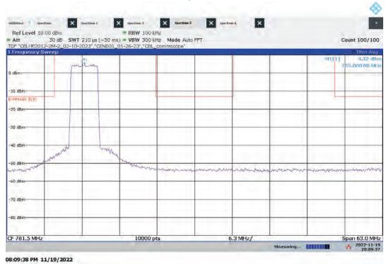
Hi-PIM – ANT1 Mid Channel Emission/Band Edge (Mask e (3)) Bandwidth: 5 MHz, Modulation: 64QAM
