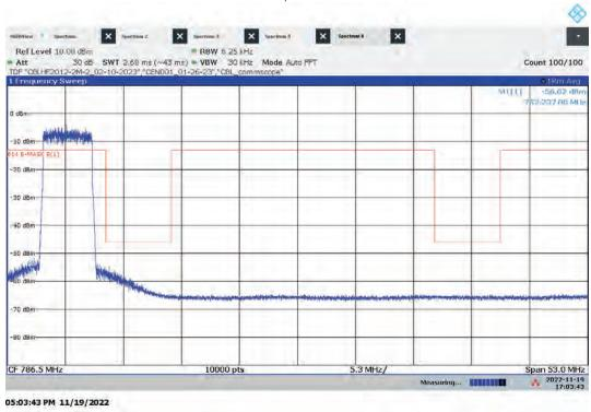
Lo-PIM – ANTO High Channel Emission/Band Edge (Mask e (3)) Bandwidth: 5 MHz, Modulation: 256QAM
