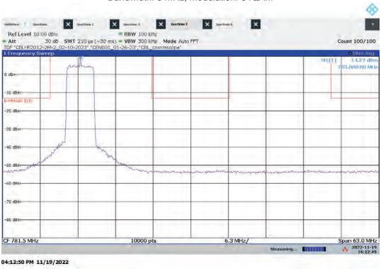
Lo-PIM – ANTO High Channel Emission/Band Edge (Mask e (1)) Bandwidth: 5 MHz, Modulation: 64QAM
