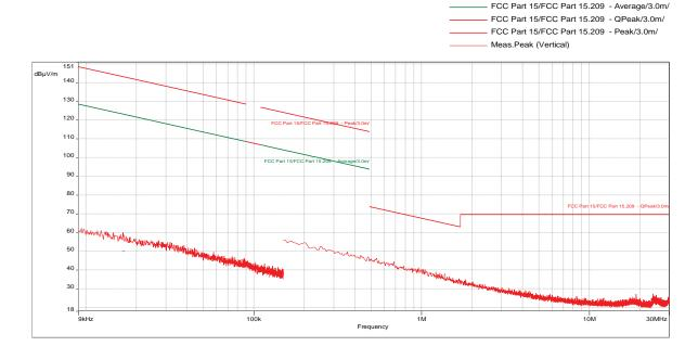
$\underline{\textbf{Results:}} \ \text{No emissions were detected above the measuring equipment noise floor}.$
