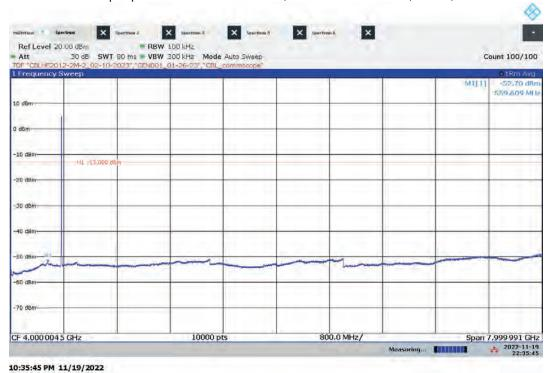
Lo-PIM Antenna Port Conducted Emissions, 9 kHz-8 GHz Worst-case output power: Bandwidth: 5 MHz, Modulation: 64QAM, ANT1, Mid Channel
