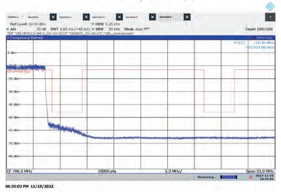
Hi-PIM – ANT1 High Channel Emission/Band Edge (Mask e (1)) Bandwidth: 10 MHz, Modulation: QPSK
