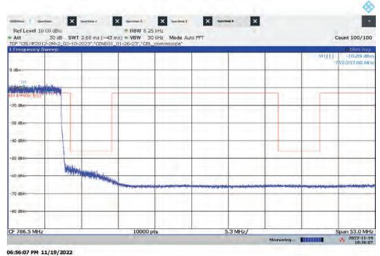
Hi-PIM – ANT1 High Channel Emission/Band Edge (Mask e (1)) Bandwidth: 10 MHz, Modulation: 256QAM
