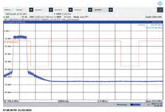
Hi-PIM – ANT1 High Channel Emission/Band Edge (Mask e (1)) Bandwidth: 5 MHz, Modulation: QPSK
