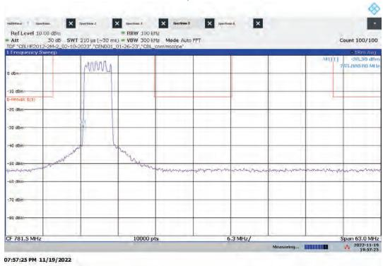
Hi-PIM – ANT0 Low Channel Emission/Band Edge (Mask e (1)) Bandwidth: 5 MHz, Modulation: 64QAM
