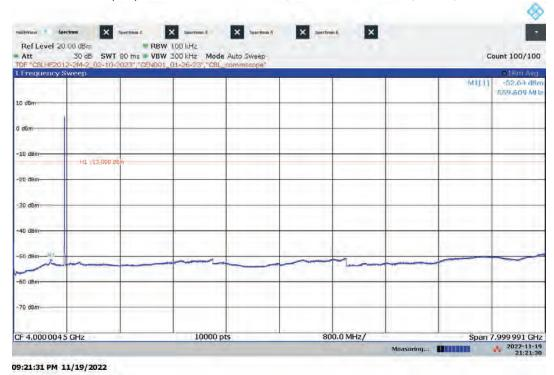
Hi-PIM Antenna Port Conducted Emissions, 9 kHz-8 GHz Worst-case output power: Bandwidth: 5 MHz, Modulation: 16QAM, ANTO, High Channel
