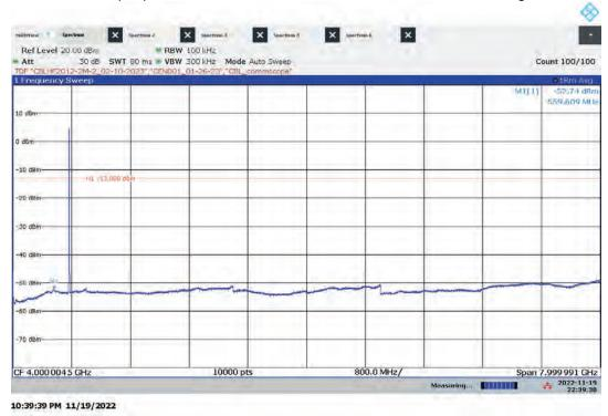
Lo-PIM Antenna Port Conducted Emissions, 9 kHz-8 GHz Worst-case output power: Bandwidth: 5 MHz, Modulation: 64QAM, ANT1, High Channel
