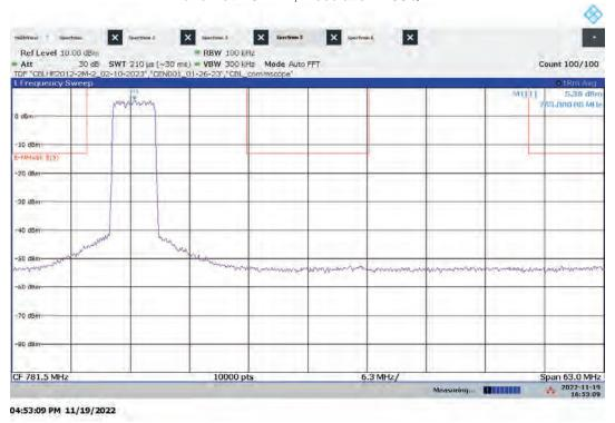
Lo-PIM – ANT1 Mid Channel Emission/Band Edge (Mask e (3)) Bandwidth: 5 MHz, Modulation: 256QAM
