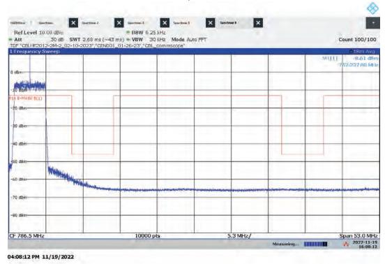
Lo-PIM – ANT1 Mid Channel Emission/Band Edge (Mask e (1)) Bandwidth: 5 MHz, Modulation: 64QAM
