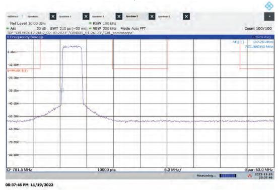
Hi-PIM – ANT1 High Channel Emission/Band Edge (Mask e (3)) Bandwidth: 5 MHz, Modulation: 256QAM
