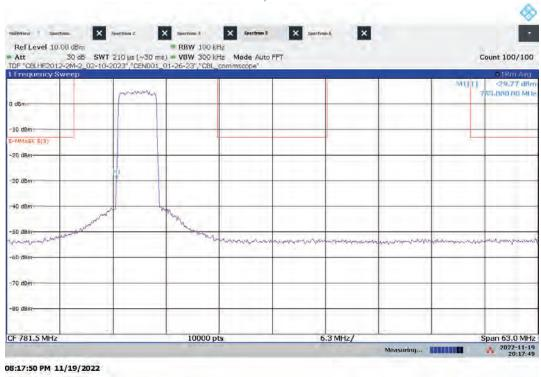
Hi-PIM – ANT0 Low Channel Emission/Band Edge (Mask e (1)) Bandwidth: 5 MHz, Modulation: 256QAM
