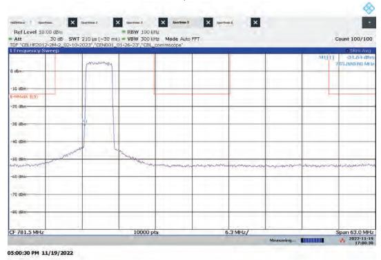
Lo-PIM – ANT1 High Channel Emission/Band Edge (Mask e (3)) Bandwidth: 5 MHz, Modulation: 256QAM
