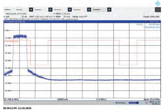
Hi-PIM – ANT1 High Channel Emission/Band Edge (Mask e (1)) Bandwidth: 5 MHz, Modulation: 256QAM
