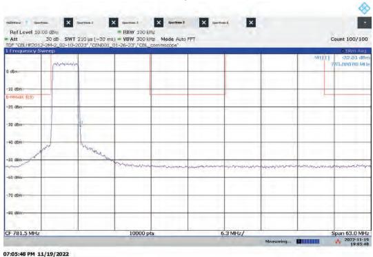
Hi-PIM – ANT1 Low Channel Emission/Band Edge (Mask e (3)) Bandwidth: 5 MHz, Modulation: QPSK
