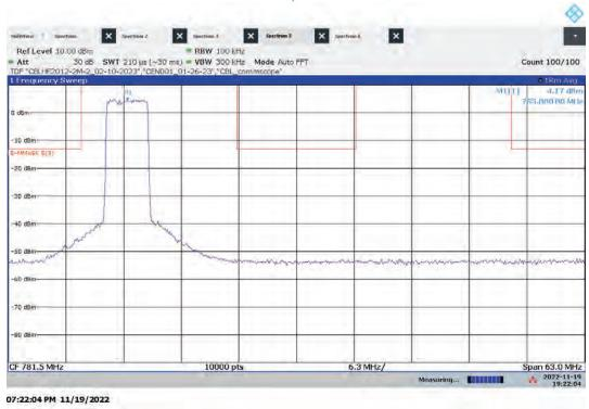
Hi-PIM – ANTO High Channel Emission/Band Edge (Mask e (1)) Bandwidth: 5 MHz, Modulation: QPSK
