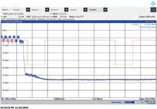
Lo-PIM – ANTO High Channel Emission/Band Edge (Mask e (3)) Bandwidth: 10 MHz, Modulation: 16QAM
