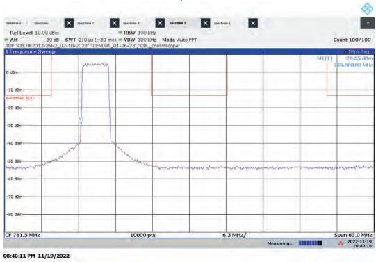
Hi-PIM – ANTO High Channel Emission/Band Edge (Mask e (1)) Bandwidth: 10 MHz, Modulation: QPSK
