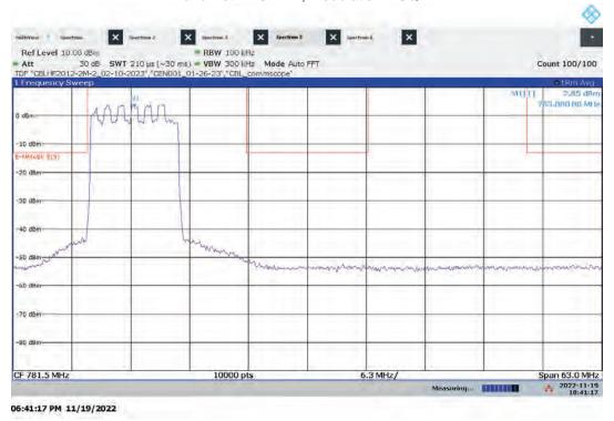
Hi-PIM – ANT1 High Channel Emission/Band Edge (Mask e (3)) Bandwidth: 10 MHz, Modulation: 16QAM
