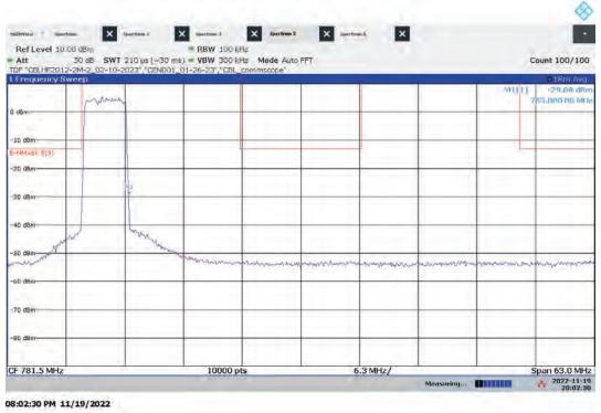
Hi-PIM – ANT1 Low Channel Emission/Band Edge (Mask e (3)) Bandwidth: 5 MHz, Modulation: 64QAM
