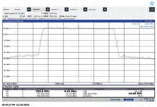
Lo-PIM – ANT1 High Channel Emission/Band Edge (Mask e (1)) Bandwidth: 10 MHz, Modulation: 64QAM
