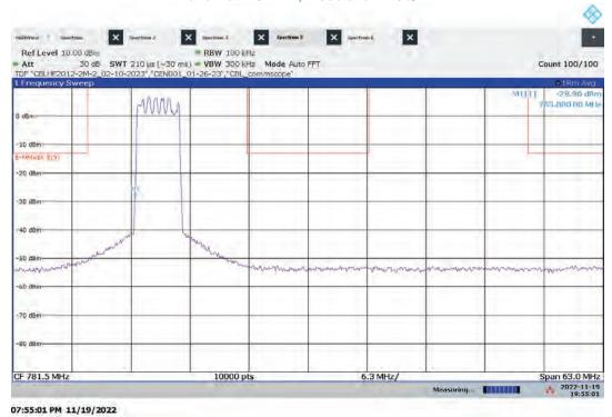
Hi-PIM – ANT1 High Channel Emission/Band Edge (Mask e (3)) Bandwidth: 5 MHz, Modulation: 16QAM
