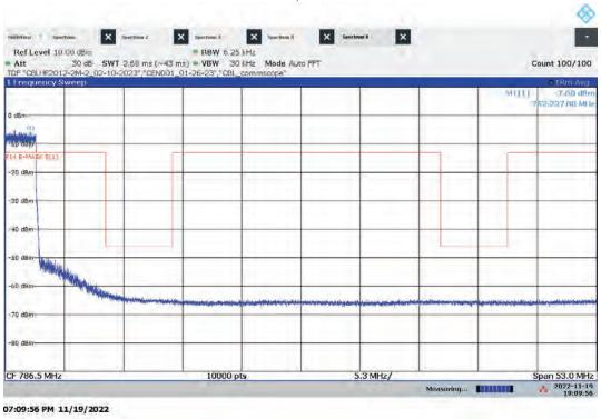
Hi-PIM – ANTO Low Channel Emission/Band Edge (Mask e (3)) Bandwidth: 5 MHz, Modulation: QPSK
