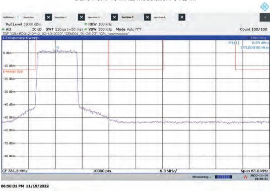
Hi-PIM – ANT0 High Channel Emission/Band Edge (Mask e (1)) Bandwidth: 10 MHz, Modulation: 256QAM
