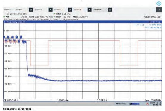
Lo-PIM – ANT1 High Channel Emission/Band Edge (Mask e (1)) Bandwidth: 10 MHz, Modulation: 16QAM
