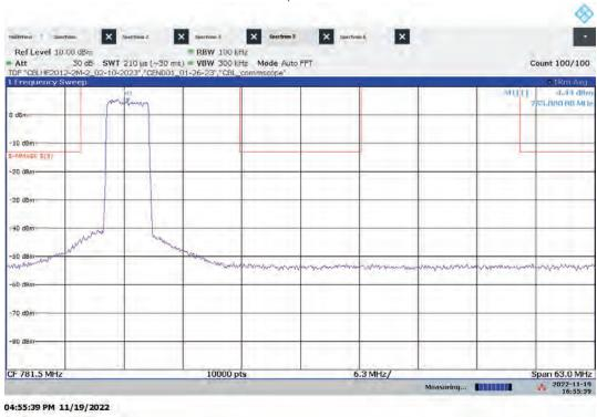
Lo-PIM – ANTO High Channel Emission/Band Edge (Mask e (1)) Bandwidth: 5 MHz, Modulation: 256QAM
