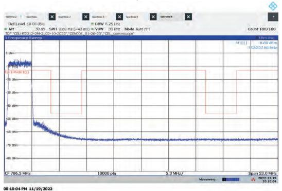
Hi-PIM – ANT1 Mid Channel Emission/Band Edge (Mask e (1)) Bandwidth: 5 MHz, Modulation: 64QAM
