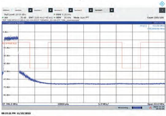
Hi-PIM – ANT0 Mid Channel Emission/Band Edge (Mask e (3)) Bandwidth: 5 MHz, Modulation: 256QAM
