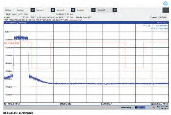
Lo-PIM – ANT1 High Channel Emission/Band Edge (Mask e (1)) Bandwidth: 5 MHz, Modulation: 256QAM
