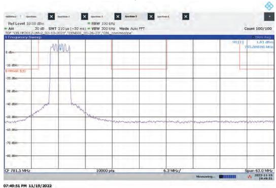
Hi-PIM – ANT1 Mid Channel Emission/Band Edge (Mask e (3)) Bandwidth: 5 MHz, Modulation: 16QAM
