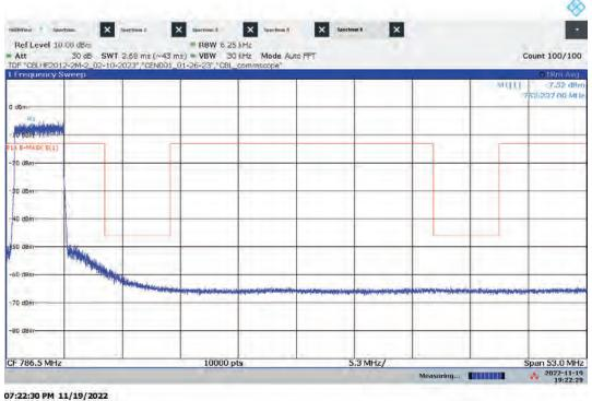
Hi-PIM – ANT0 Mid Channel Emission/Band Edge (Mask e (3)) Bandwidth: 5 MHz, Modulation: QPSK
