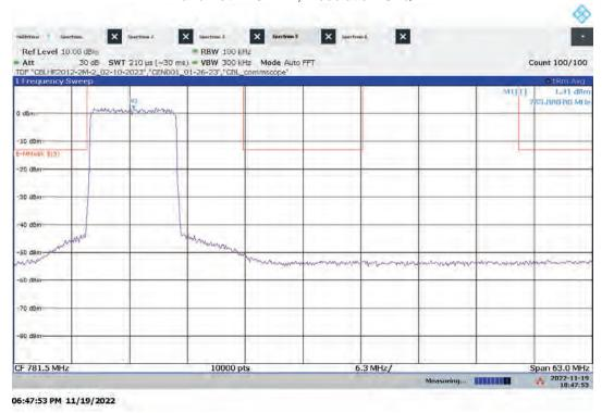
Hi-PIM – ANT1 High Channel Emission/Band Edge (Mask e (3)) Bandwidth: 10 MHz, Modulation: 64QAM
