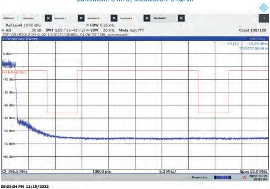
Hi-PIM – ANT0 Low Channel Emission/Band Edge (Mask e (3)) Bandwidth: 5 MHz, Modulation: 64QAM
