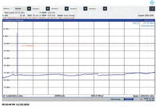
> Hi-PIM Radiated Emissions, 9 kHz-30 MHz Worst-case output power: Bandwidth: 5 MHz, Modulation: 16QAM, Low Channel (Only low channel was selected for testing in this frequency range)
