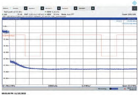
Hi-PIM – ANT1 Low Channel Emission/Band Edge (Mask e (1)) Bandwidth: 5 MHz, Modulation: 64QAM
