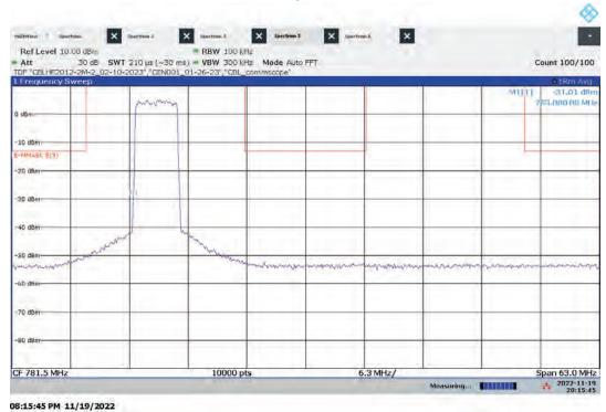
Hi-PIM – ANT1 High Channel Emission/Band Edge (Mask e (3)) Bandwidth: 5 MHz, Modulation: 64QAM
