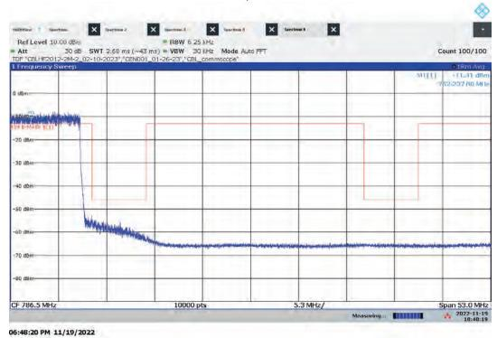
Hi-PIM – ANT1 High Channel Emission/Band Edge (Mask e (1)) Bandwidth: 10 MHz, Modulation: 64QAM
