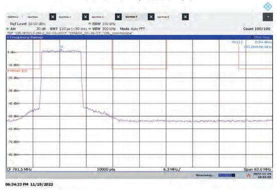
Hi-PIM – ANT1 High Channel Emission/Band Edge (Mask e (3)) Bandwidth: 10 MHz, Modulation: QPSK
