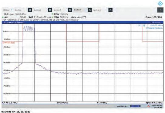
Hi-PIM – ANT1 Low Channel Emission/Band Edge (Mask e (3)) Bandwidth: 5 MHz, Modulation: 16QAM
