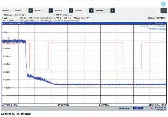
Hi-PIM – ANT0 High Channel Emission/Band Edge (Mask e (3)) Bandwidth: 10 MHz, Modulation: 256QAM
