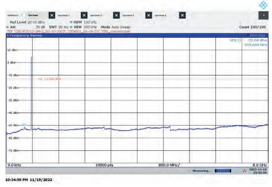
Lo-PIM Antenna Port Conducted Emissions, 9 kHz-8 GHz Worst-case output power: Bandwidth: 5 MHz, Modulation: 64QAM, ANTO, High Channel
