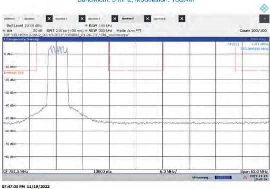
Hi-PIM – ANTO High Channel Emission/Band Edge (Mask e (1)) Bandwidth: 5 MHz, Modulation: 16QAM
