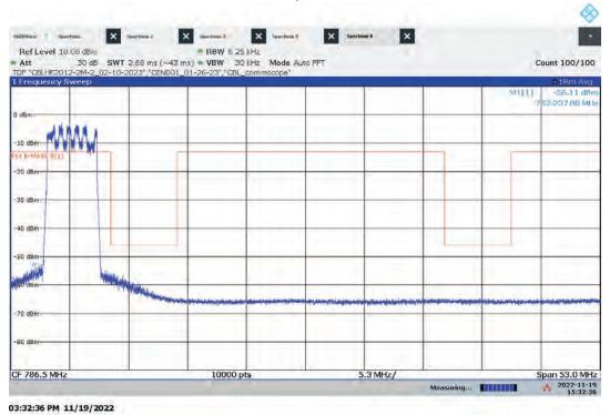
Lo-PIM – ANT1 High Channel Emission/Band Edge (Mask e (1)) Bandwidth: 5 MHz, Modulation: 16QAM
