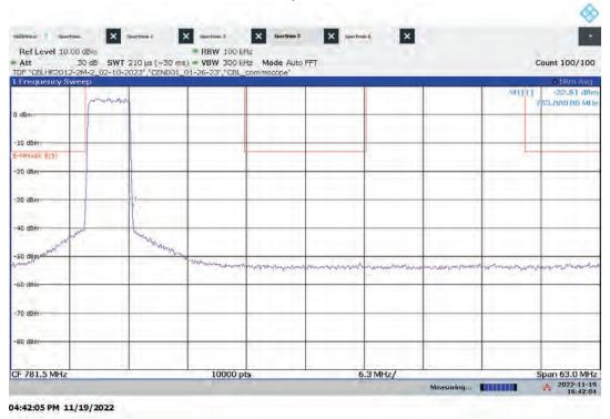
Lo-PIM – ANT1 Low Channel Emission/Band Edge (Mask e (3)) Bandwidth: 5 MHz, Modulation: 256QAM
