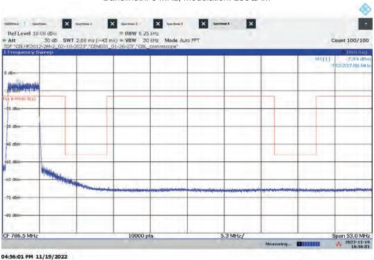
Lo-PIM – ANTO Mid Channel Emission/Band Edge (Mask e (3)) Bandwidth: 5 MHz, Modulation: 256QAM
