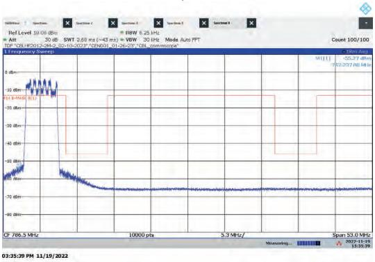
Lo-PIM – ANTO High Channel Emission/Band Edge (Mask e (3)) Bandwidth: 5 MHz, Modulation: 16QAM
