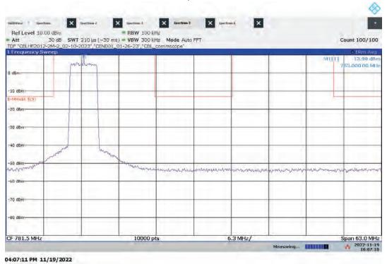
Lo-PIM – ANT1 Mid Channel Emission/Band Edge (Mask e (3)) Bandwidth: 5 MHz, Modulation: 64QAM
