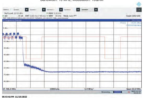
Hi-PIM – ANTO High Channel Emission/Band Edge (Mask e (3)) Bandwidth: 10 MHz, Modulation: 16QAM
