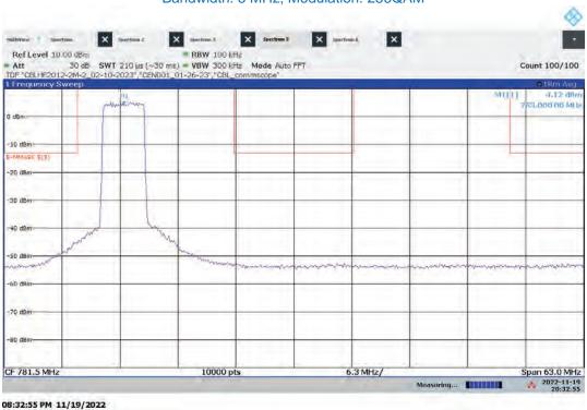
Hi-PIM – ANTO High Channel Emission/Band Edge (Mask e (1)) Bandwidth: 5 MHz, Modulation: 256QAM
