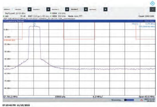
Hi-PIM – ANT1 Mid Channel Emission/Band Edge (Mask e (3)) Bandwidth: 5 MHz, Modulation: QPSK
