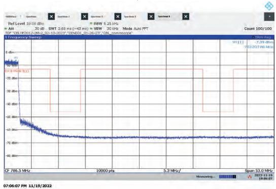
Hi-PIM – ANT1 Low Channel Emission/Band Edge (Mask e (1)) Bandwidth: 5 MHz, Modulation: QPSK
