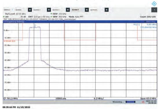
Hi-PIM – ANT1 Mid Channel Emission/Band Edge (Mask e (3)) Bandwidth: 5 MHz, Modulation: 256QAM
