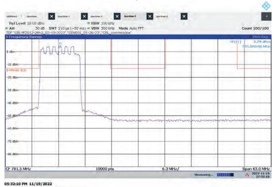
Lo-PIM – ANT1 High Channel Emission/Band Edge (Mask e (3)) Bandwidth: 10 MHz, Modulation: 16QAM
