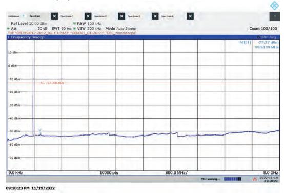
Hi-PIM Antenna Port Conducted Emissions, 9 kHz-8 GHz Worst-case output power: Bandwidth: 5 MHz, Modulation: 16QAM, ANT1, Low Channel
