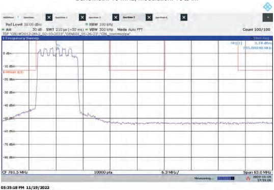
Lo-PIM – ANTO High Channel Emission/Band Edge (Mask e (1)) Bandwidth: 10 MHz, Modulation: 64QAM
