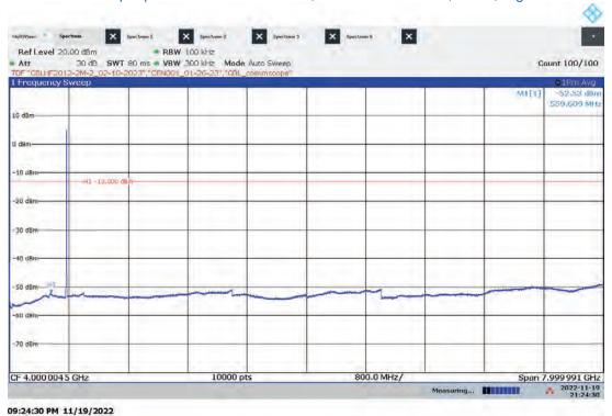
Hi-PIM Antenna Port Conducted Emissions, 9 kHz-8 GHz Worst-case output power: Bandwidth: 5 MHz, Modulation: 16QAM, ANT1, High Channel
