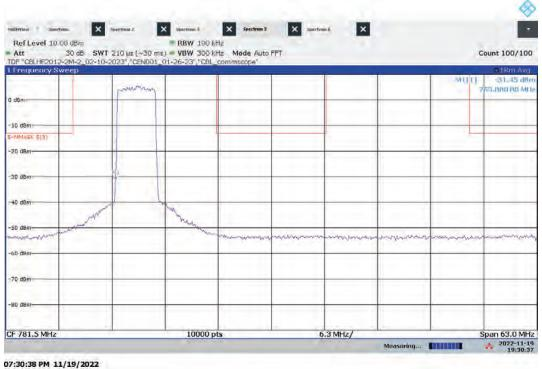
Hi-PIM – ANT0 Low Channel Emission/Band Edge (Mask e (1)) Bandwidth: 5 MHz, Modulation: 16QAM
