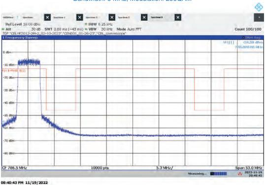
Hi-PIM – ANTO High Channel Emission/Band Edge (Mask e (3)) Bandwidth: 5 MHz, Modulation: 256QAM
