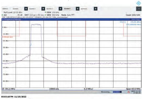
Lo-PIM – ANTO High Channel Emission/Band Edge (Mask e (1)) Bandwidth: 10 MHz, Modulation: QPSK
