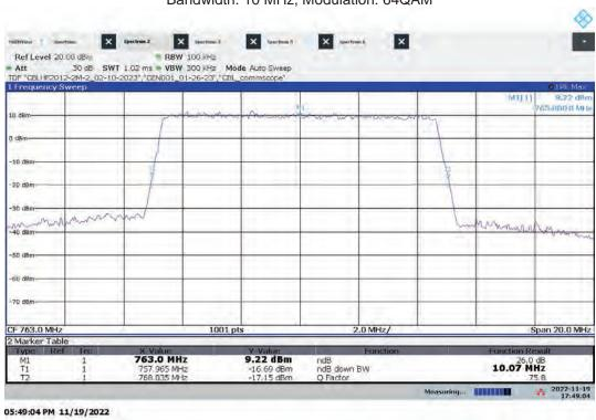
Lo-PIM – ANTO High Channel Emission/Band Edge (Mask e (3)) Bandwidth: 10 MHz, Modulation: 64QAM
