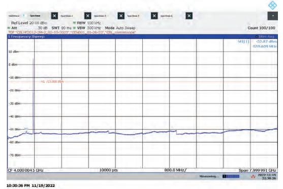
Lo-PIM Antenna Port Conducted Emissions, 9 kHz-8 GHz Worst-case output power: Bandwidth: 5 MHz, Modulation: 256QAM, ANT1, Low Channel
