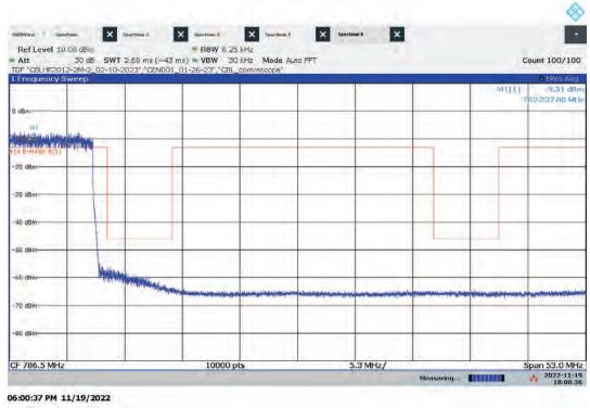
Lo-PIM – ANTO High Channel Emission/Band Edge (Mask e (3)) Bandwidth: 10 MHz, Modulation: 256QAM
