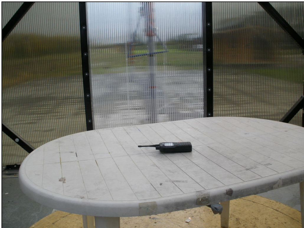
Photograph 3 Standalone: Radiated Emissions - Flat
