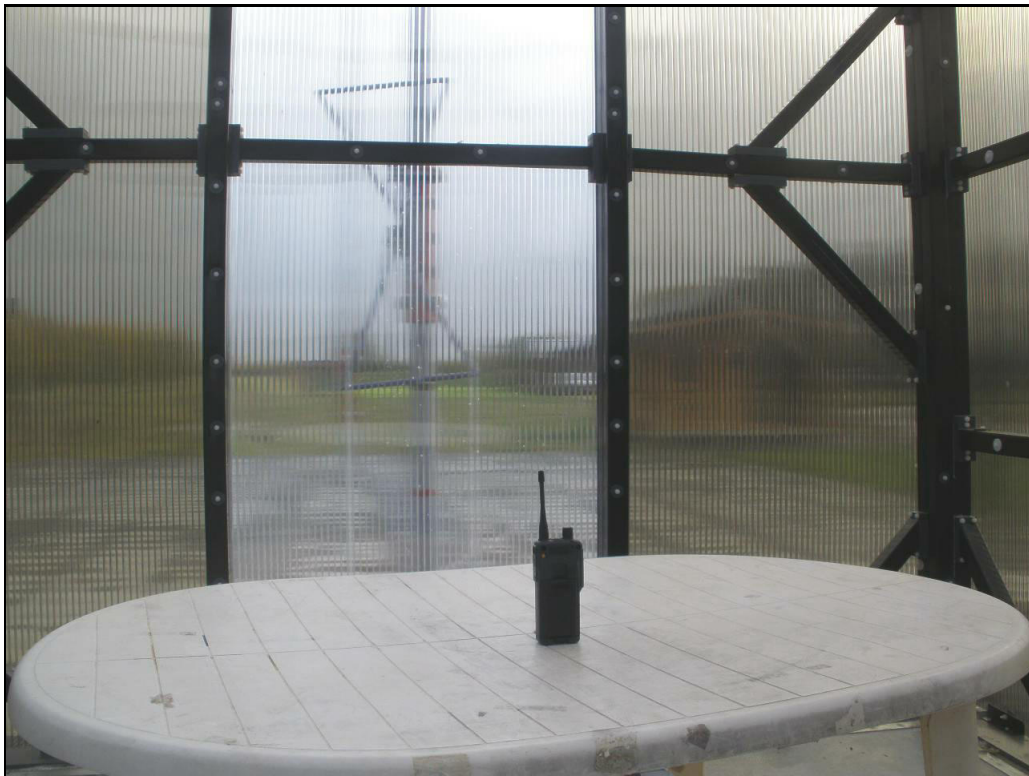
Photograph 2 Standalone: Radiated Emissions - Upright
