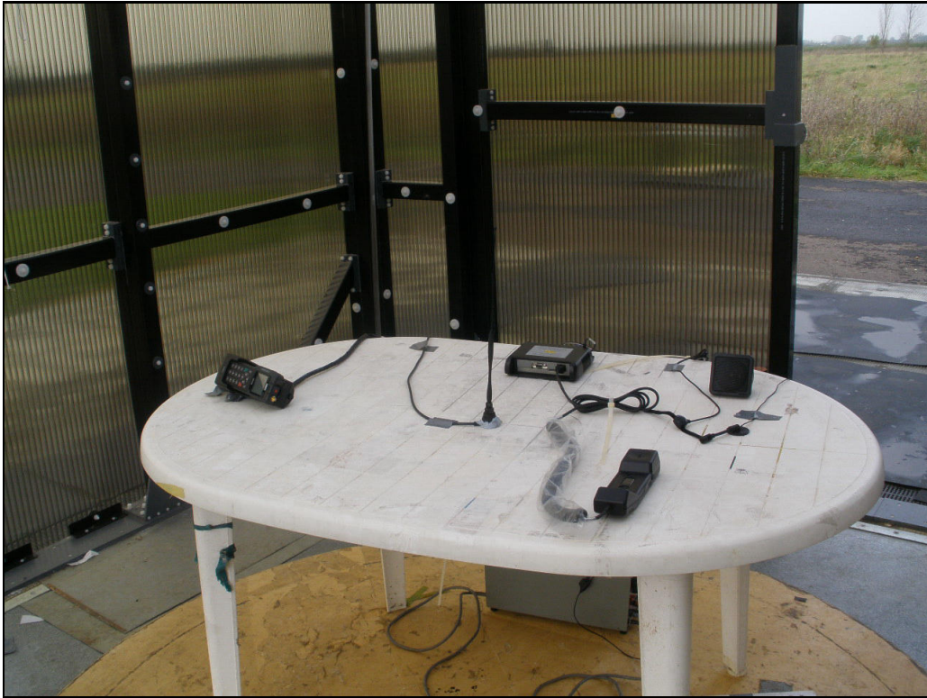
Photograph 6 Car Kit: Radiated Emissions - Front
