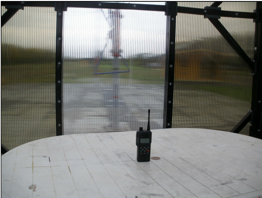
Photograph 8 STP9280: Radiated Emissions - Front
