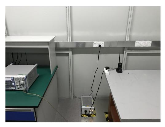
**RADIATED EMISSION TEST SETUP**
