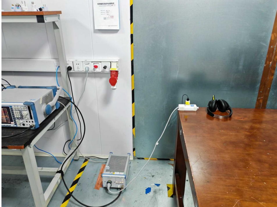
Conducted emissions at AC power line (150kHz-30MHz)
