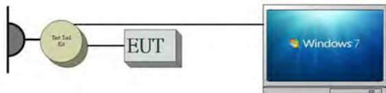
Fig 2-2 Conducted (Antenna Port) Configuration
