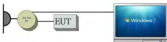
Fig 2-2 Conducted (Antenna Port) Configuration
