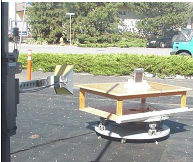
Photograph B.7-2 - Horn Receive Antenna with DUT Antenna - DUT "Portrait" Configuration
