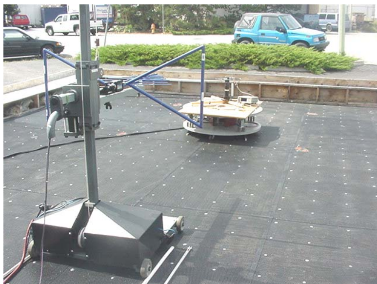
Photograph B.7-3 - Dipole Substitution Setup
