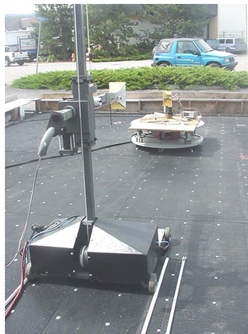
Photograph B.7-4 - Horn Substitution Setup
