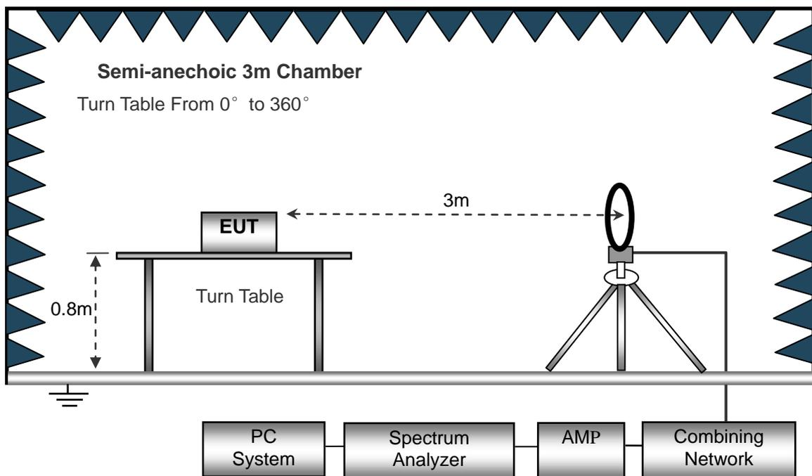
The test setup for emission measurement from 30MHz to 1GHz.
