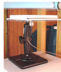
SAR Test Setup – 2.5cm spacing with Tecom Patch Antenna
