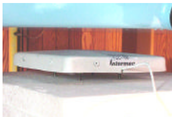
SAR Test Setup – 2.0cm spacing with Mobile Mark Patch Antenna
