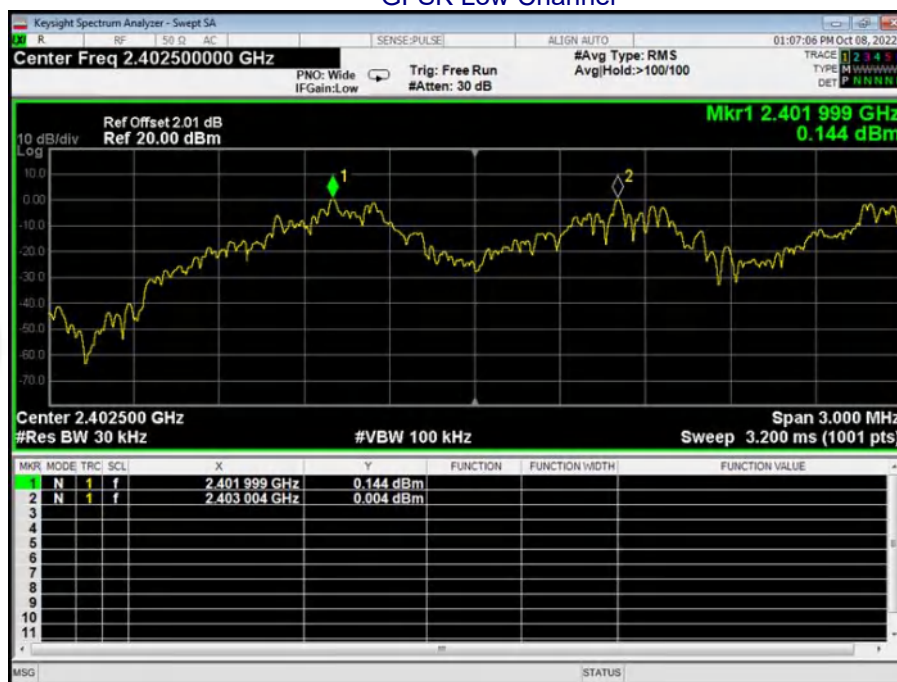
Test plots GFSK Low Channel
