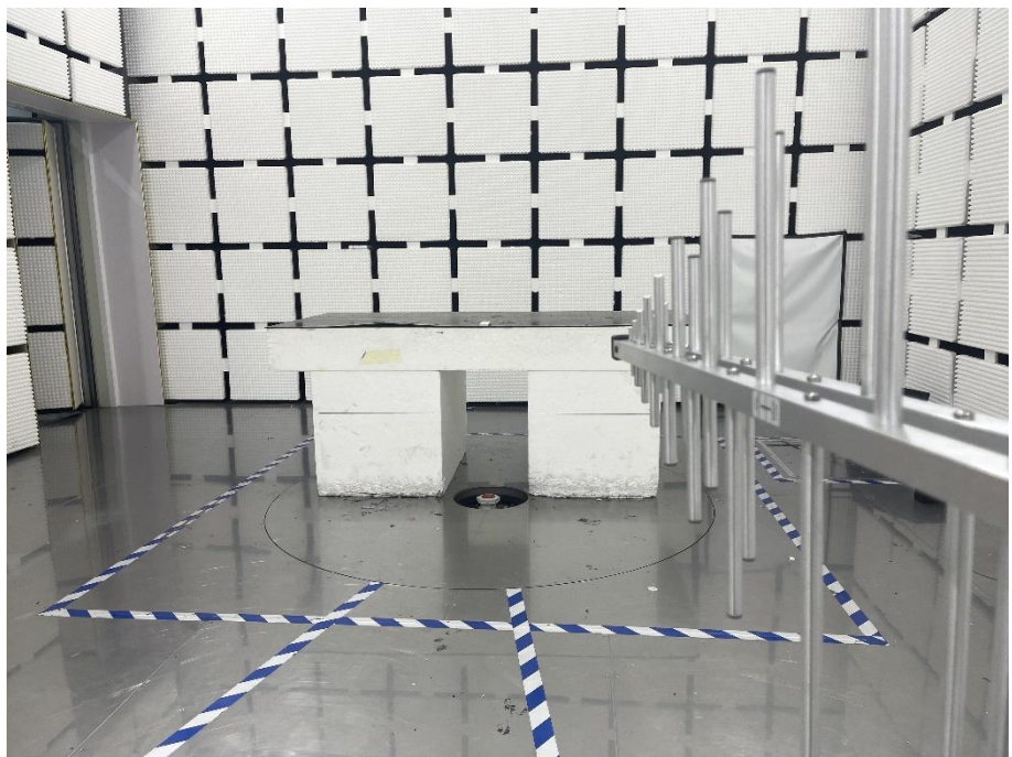
Radiation Emission Test Setup (30MHz to 1GHz)
