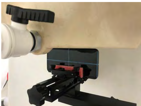
Fig.19 EUT Left side to flat phantom
