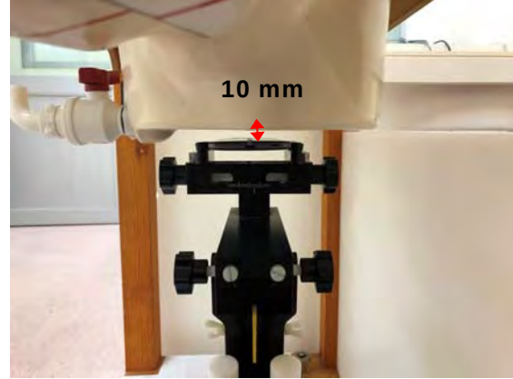
Fig.9 EUT Front side to flat phantom
