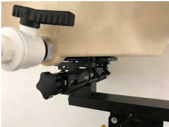
Fig.16 EUT Back side to flat phantom
