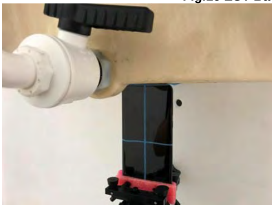
Fig.17 EUT Top side to flat phantom
