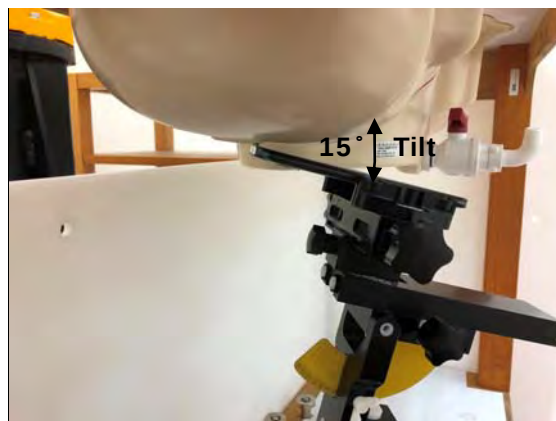
Fig.4 Right Head Section / Ear-Tilt Position(15°)
