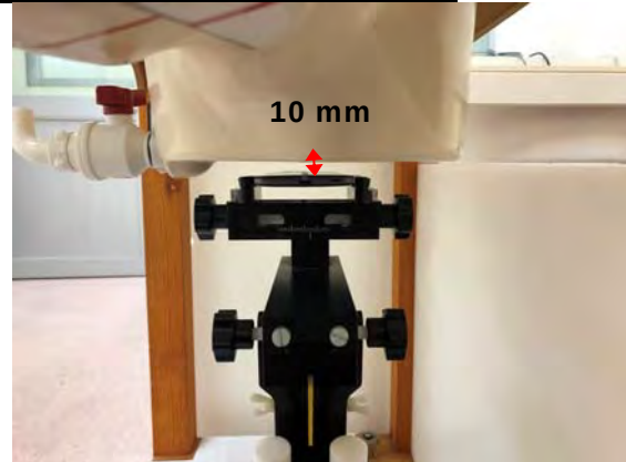
Fig.7 EUT Front side to flat phantom
