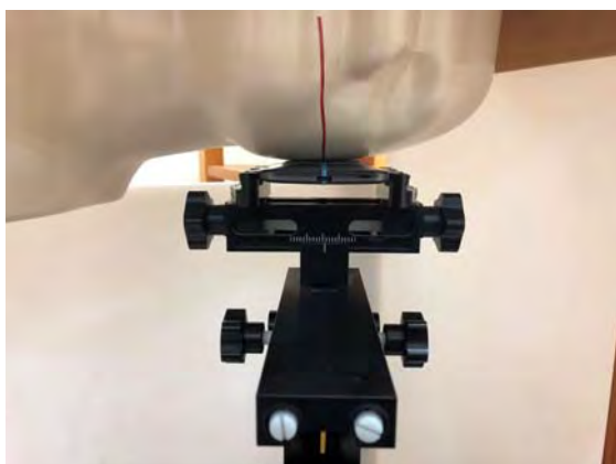
Fig.5 Left Head Section / Cheek-Touch Position
