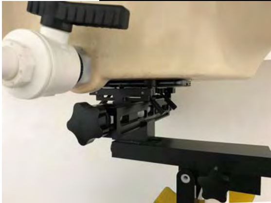
Fig.15 EUT Front side to flat phantom
