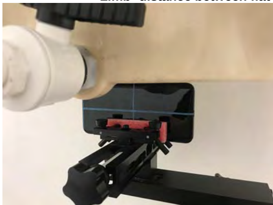
Fig.18 EUT Right side to flat phantom
