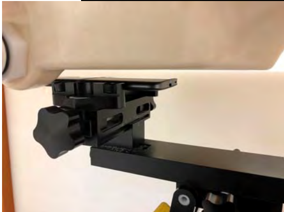
Fig.7 EUT Front side to flat phantom
