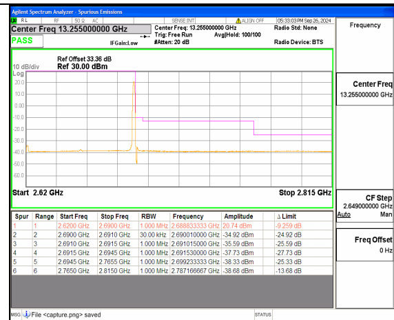
n41 70M DFT-s-OFDM QPSK Edge_1RB_Right High
