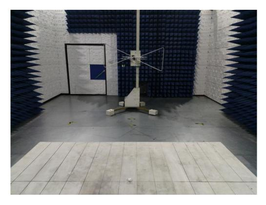
RADIATED EMISSION TEST SETUP ABOVE 1GHZ
