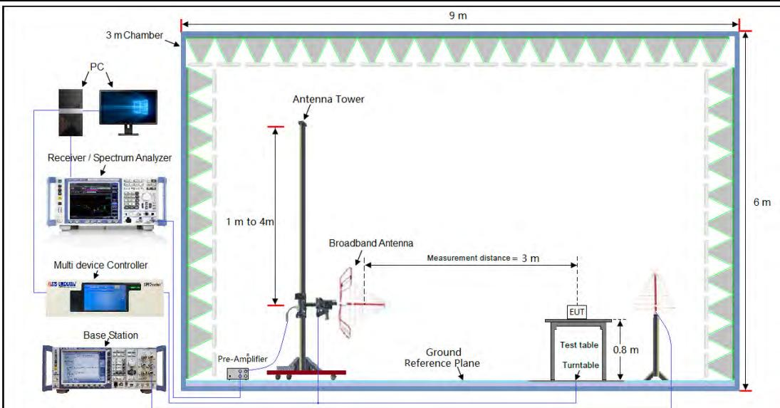
Radiated Emissions Above 1GHz Test setup
