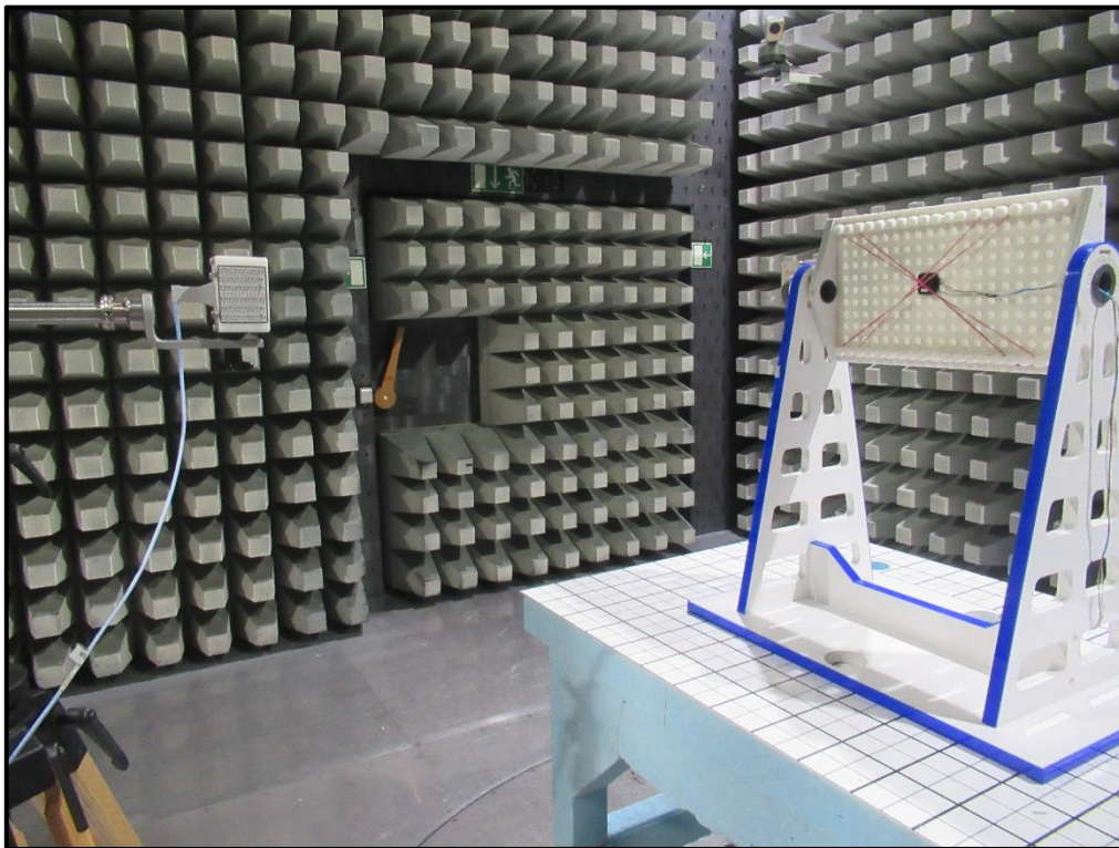
Photo 7: Radiated Test Setup-18 GHz – 25 GHz
