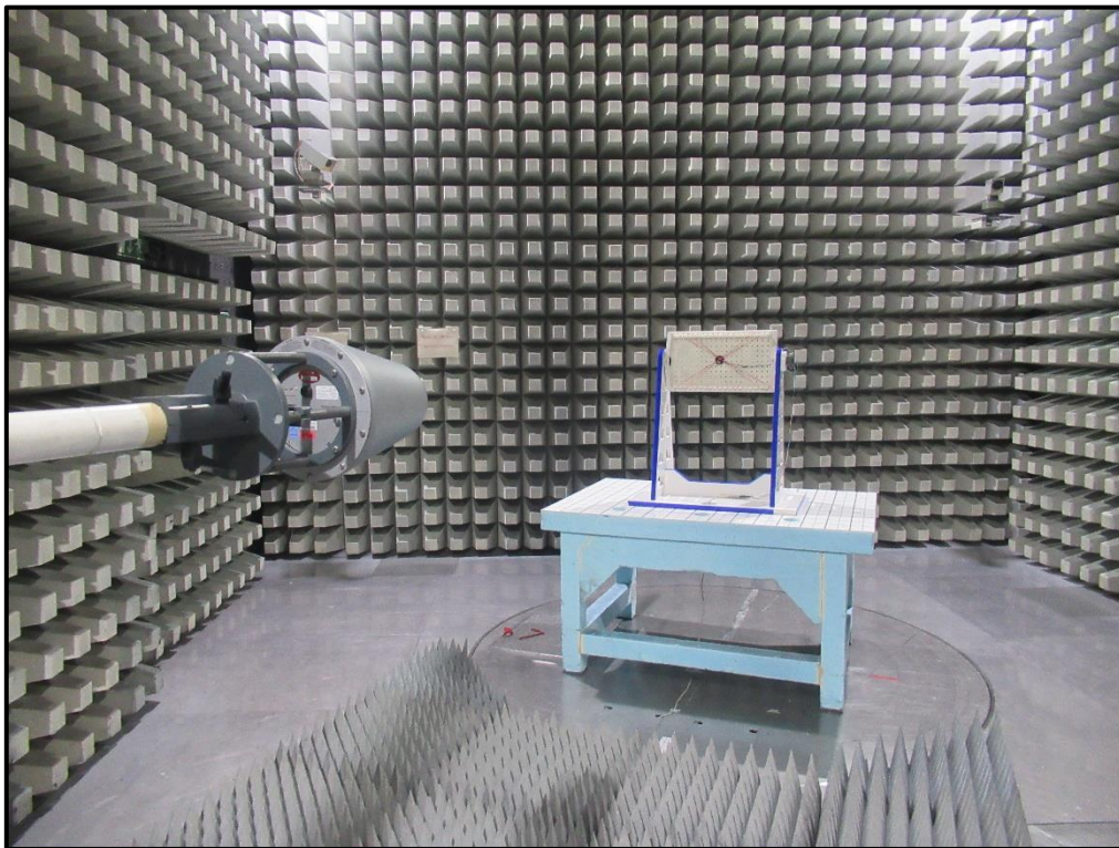
Photo 5: Radiated Test Setup-1 GHz to 18 GHz
