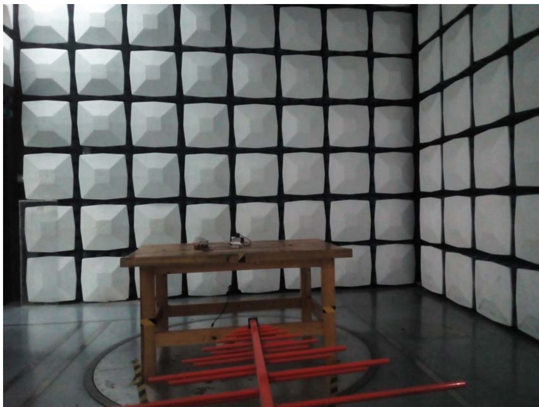
Radiated Emission Above 1GHz View
