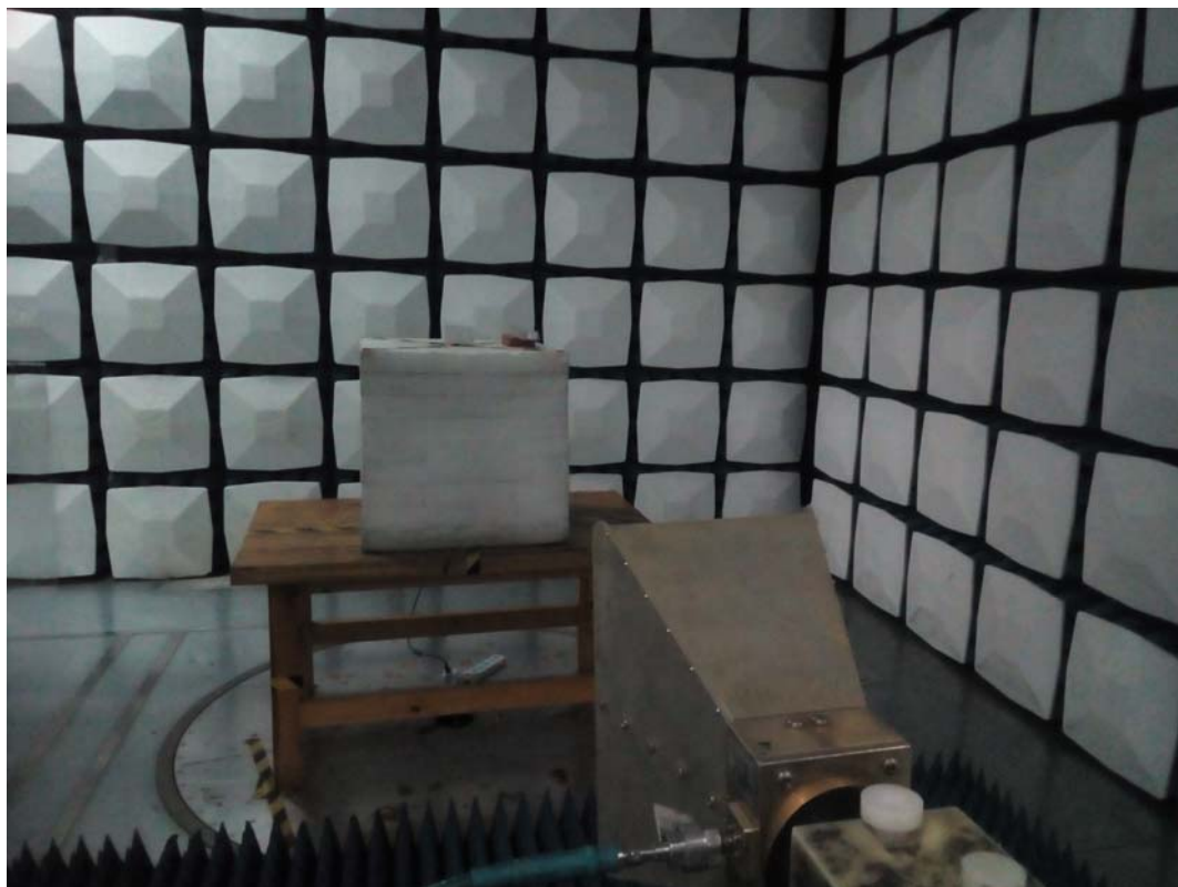
Radiated Emission Above 1GHz View
