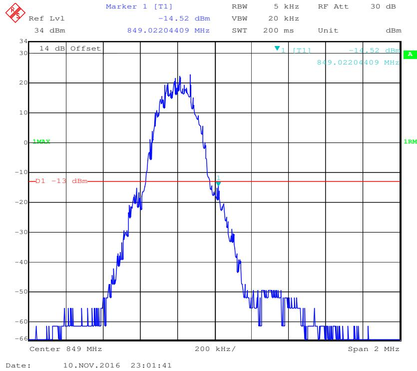
**Cellular Band, Left Band Edge for WCDMA (BPSK) Mode**
