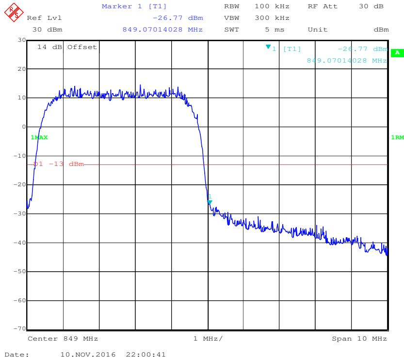
**Cellular Band, Left Band Edge for HSUPA (BPSK) Mode**
