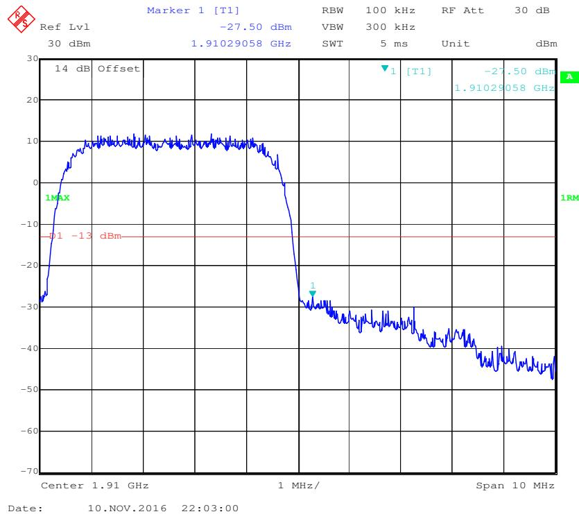
**PCS Band, Left Band Edge for HSUPA (BPSK) Mode**
