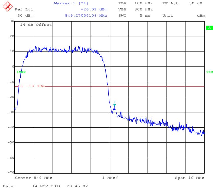
**PCS Band, Left Band Edge for GSM (GMSK) Mode**
