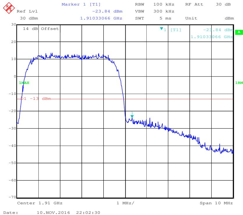
**PCS Band, Left Band Edge for HSDPA (16QAM) Mode**
