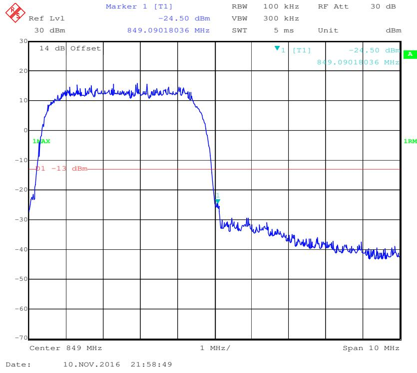
**Cellular Band, Left Band Edge for HSDPA (16QAM) Mode**
