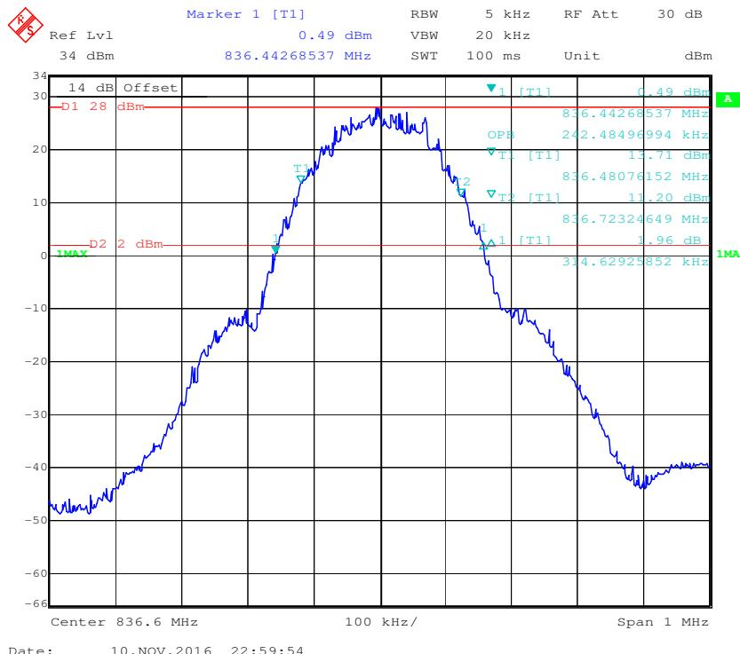
**99% Occupied Bandwidth & 26 dB Emissions Bandwidth for RMC (BPSK) Mode**
