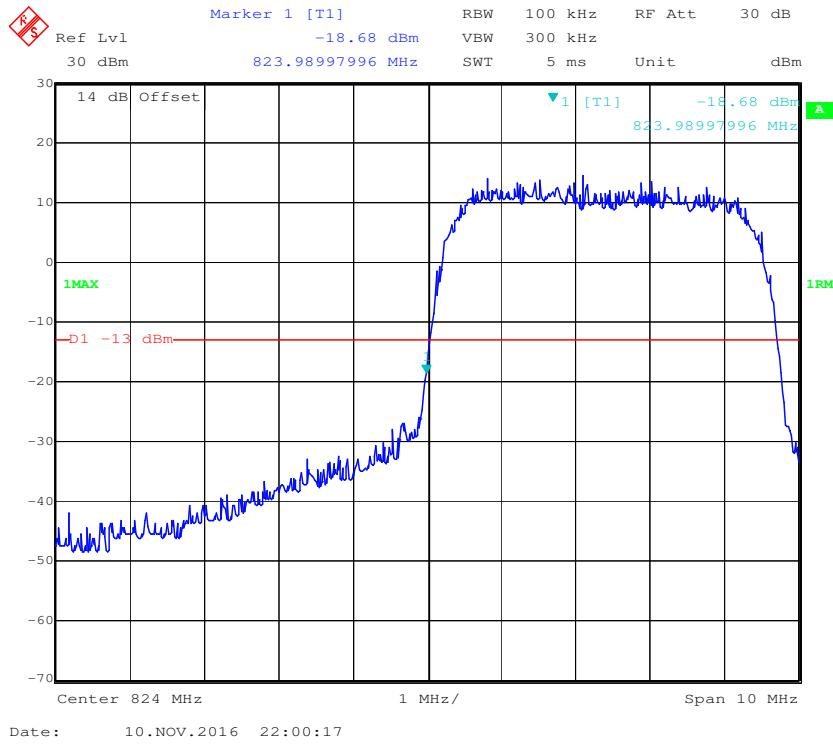
**Cellular Band, Right Band Edge for HSDPA (16QAM) Mode**
